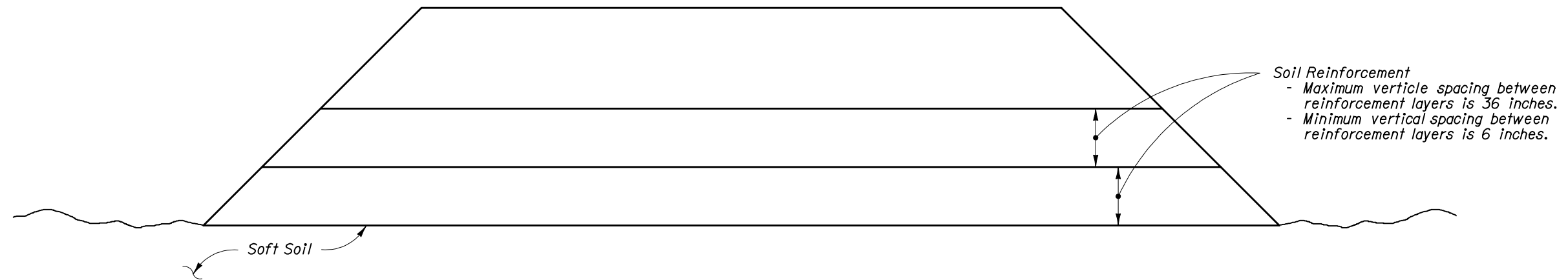
GEOSYNTHETIC REINFORCED FOUNDATIONS CONSTRUCTED ON SOFT SOILS
