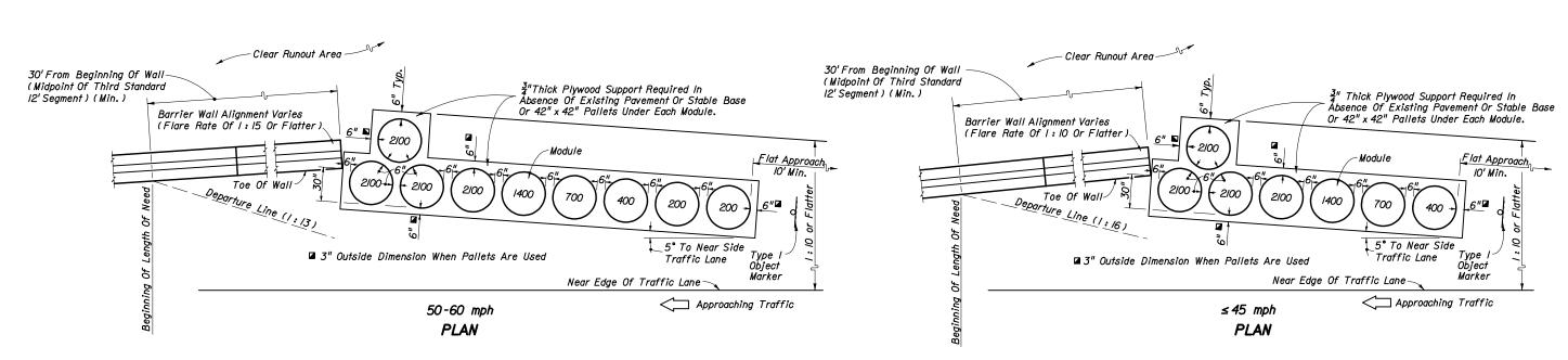
Note: Numbers shown inside modules indicate mass in pounds of sand. All modules are approximately 3' in diameter with heights ranging from 3' to 3'-9".
