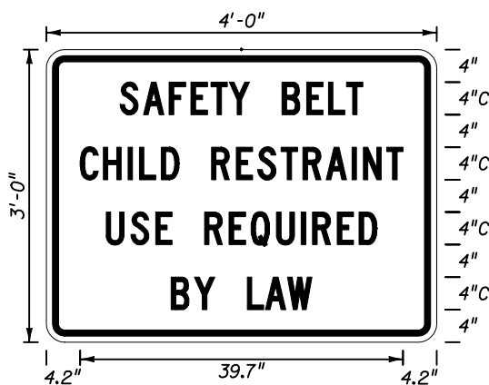
FTP-45-04 4' X 3' 1 1/2" Radii 3/4" Border 4" Series C Legend White Background Black Legend & Border
