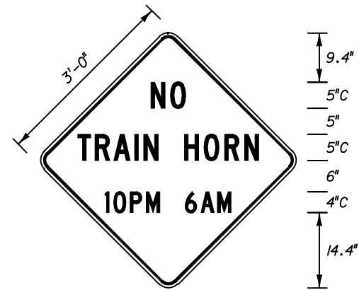
FTP-62-04 3' X 3' Series C Legend 2" Radii \frac{3}{4} " Border Yellow Background Black Legend & Border
