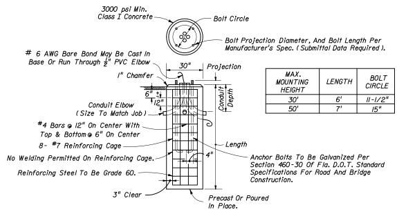
METAL POLE CONCRETE FOUNDATION DETAIL
