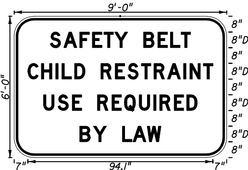
FTP-44-04 9' X 6' 9" Radii 3/4" Border 8" Series D Legend White Background Black Legend & Border
