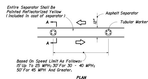
Notes: (a) The tubular marker is to be made of a flexible material or have a flexible joint at the base such that it will not cause damage to vehicles upon impact and will return to its original shape after being struck by a 5000 lb. vehicle at a velocity of 75'/sec.
