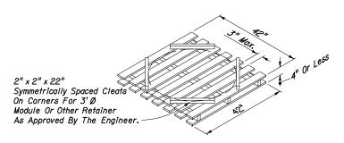
Pallet Shall Be Constructed Of Wood Or Other Frangible Or Resilient Materials Other Than Metals, And, Shall Be Sufficiently Durable To Support Modules For Their Expected Period Of Use; Wood Pallet Detail Shown.
