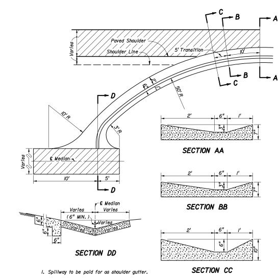
2. If spillway empties into a shallow or median ditch, the detail should be modified as necessary.
