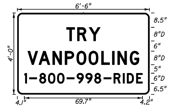
FTP - 64 6'-6" X 4' 3" Radii 8" Series D 6" Series D Blue Background White Legend & Border
