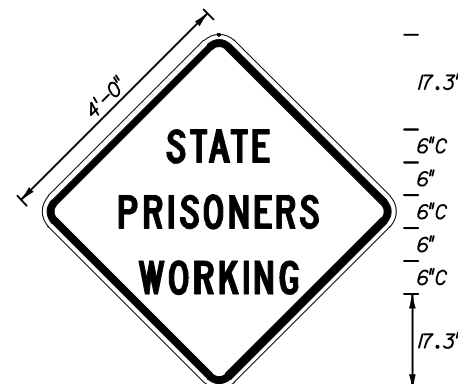
MOT - 11 4' X 4' 3" Radii 3/4" Border 6" Series C Legend Orange Background Black Legend & Border
