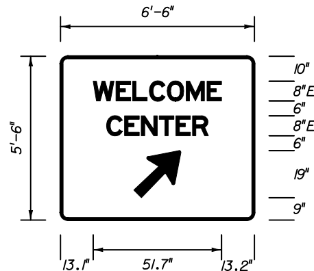
FTP - 20 6'-6" X 5'-6" 3" Radii 2" Border Series E Legend Blue Background White Legend & Border
