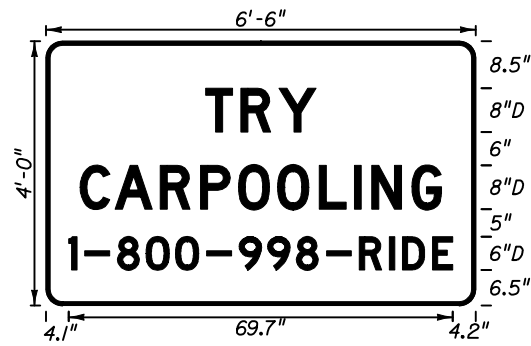
FTP - 68 6'-6" X 4' 3" Radii 8" Series D 6" Series D Blue Background White Legend & Border
