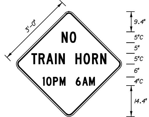
FTP - 38B 3' X 3' Series C Legend 2" Radii 3/4" Border Yellow Background Black Legend & Border
