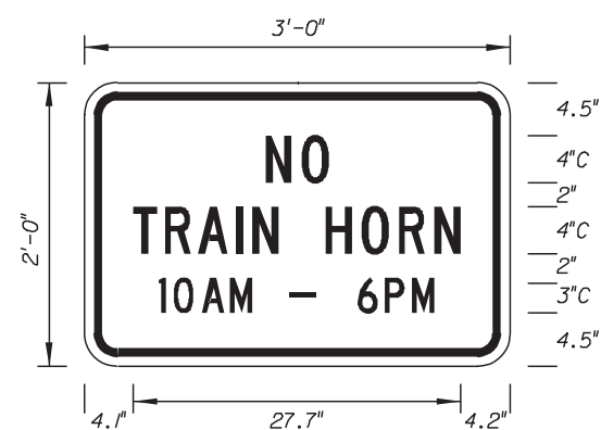
FTP - 38A 3' X 2' Series C Legend 2" Radii 3/4" Border Yellow Background Black Legend & Border
