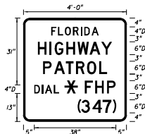
FTP - 62 4' x 4' 3" Radii 1" Border Series D Blue Background White Legend & Border
