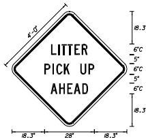
MOT - 4 4' x 4' 3" Radii 3/4" Border Orange Background Black Arrows & Border
