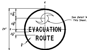
FTP - 53 2' Diameter \frac{3}{4} " Border 3" Series C Blue Background White Legend - Border & Symbol
