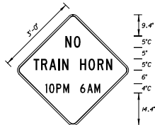
FTP - 38B 3' X 3' Series C Legend 2" Radii 3/4" Border Yellow Background Black Legend & Border
