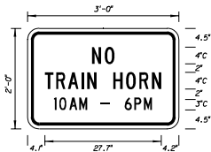
FTP - 38A 3' X 2' Series C Legend 2" Radii 3/4" Border Yellow Background Black Legend & Border
