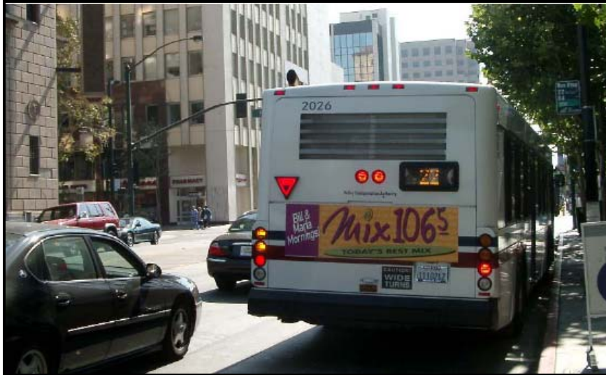
Figure 22 Santa Clara Valley Transportation Authority Bus with LED Yield Sign (Source: TCRP Synthesis 49)
