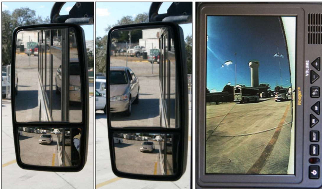
Figure 5-31. Mirror views for vehicle located behind the length of the bus
