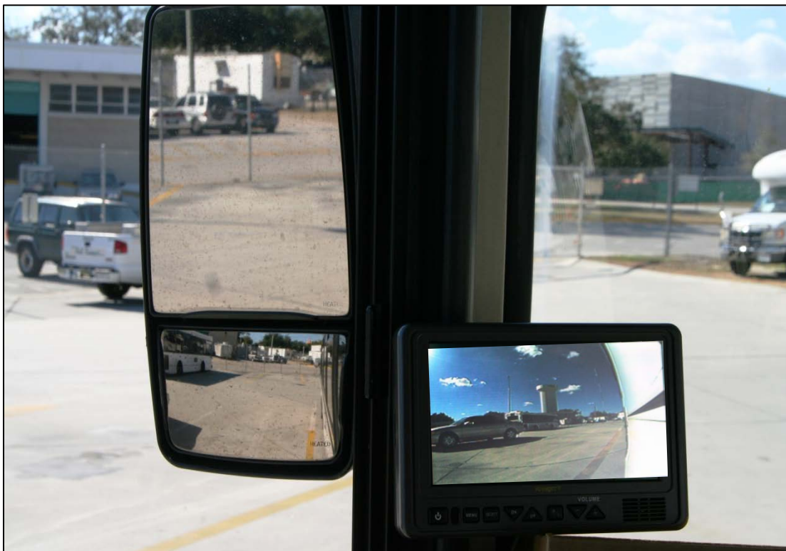
Figure 5-4. Vehicle visible with video system but not with mirrors
