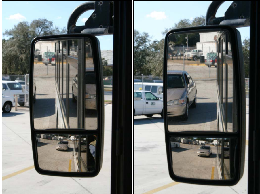
Figure 2-13. Mirror views for vehicle located behind the length of the bus
