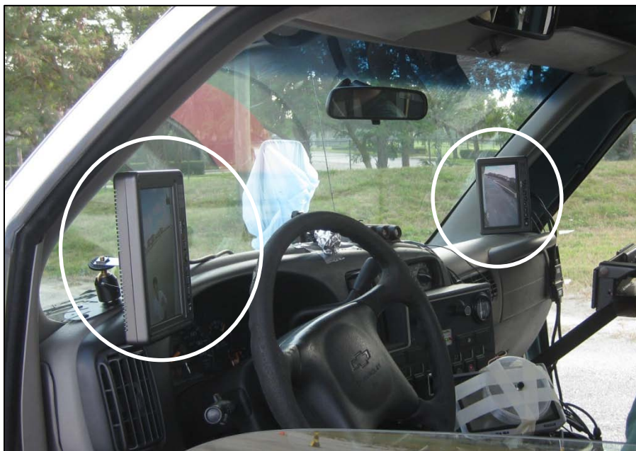
Figure 2-8. Two monitors installed on driver's dashboard
