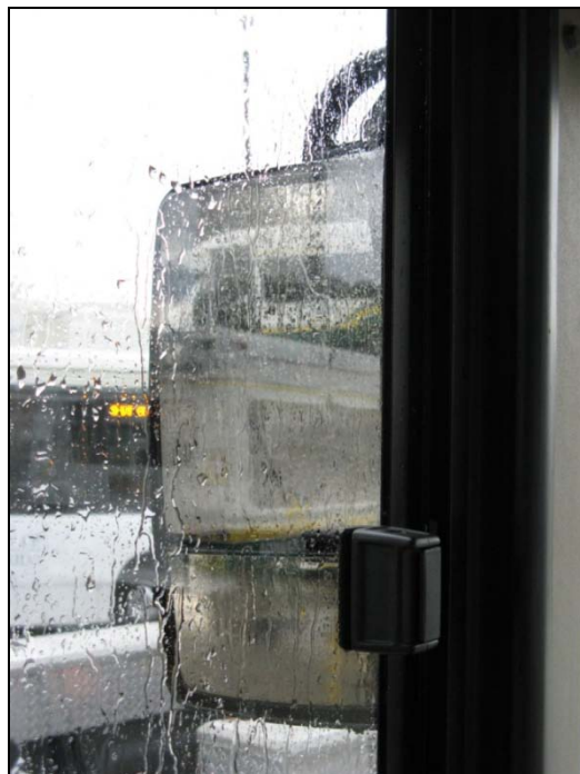
Figure 5-29. Image from mirror through driver's window while raining
