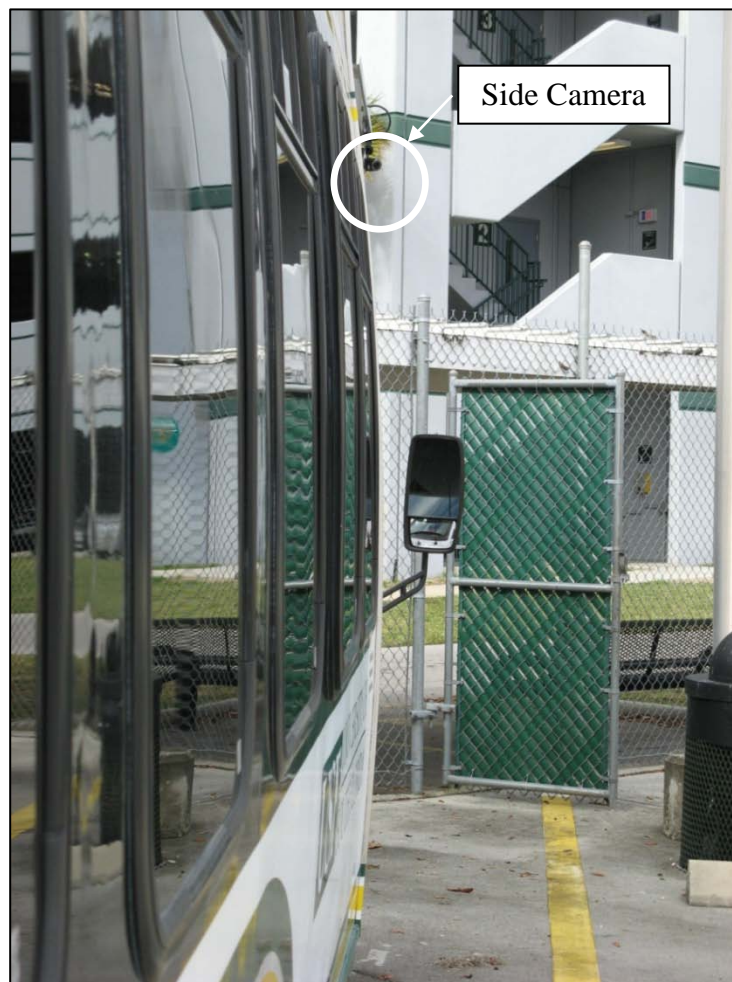
Figure 5-32. Side camera location on cutaway bus
