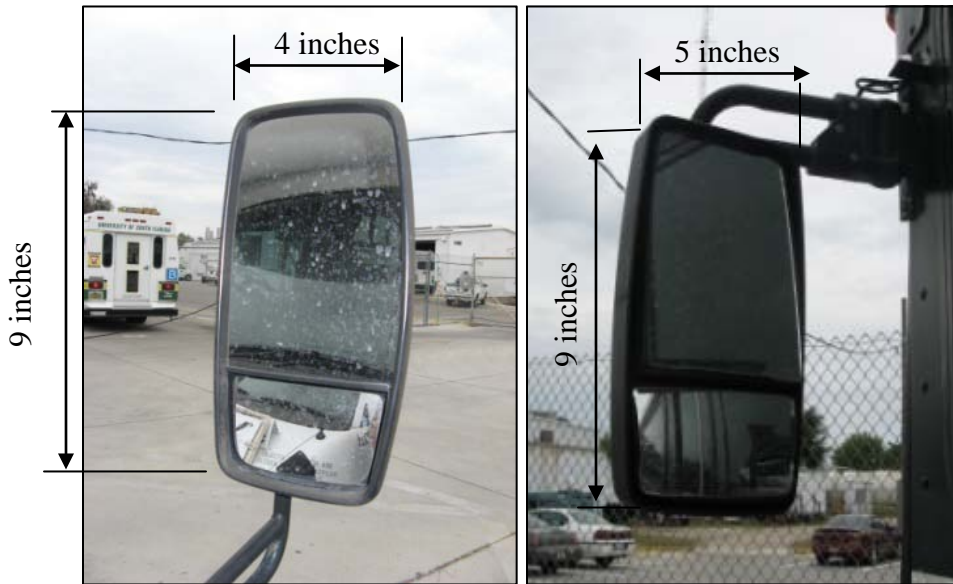
Figure 2-3. Different types of mirror-based systems
