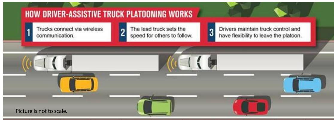
The driver in the leader truck drives normally, controlling throttle, brakes, and steering. The driver in the follower truck allows the system to control throttle and brakes while he or she retains responsibility for steering and monitoring/responding to the driving environment; the human driver continues to play an essential role in the driving task.
