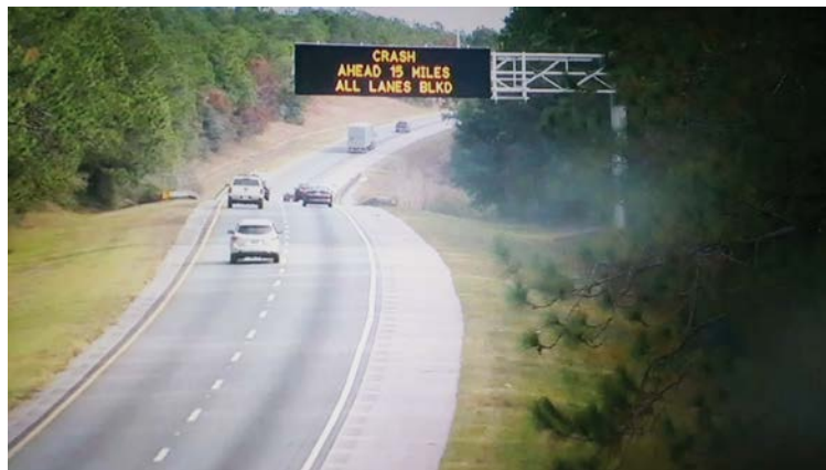
Message on dynamic message sign alerting travelers of blocked lanes.
