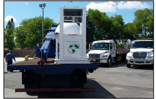
Propane fuel station installed to support Road Ranger fleet.
