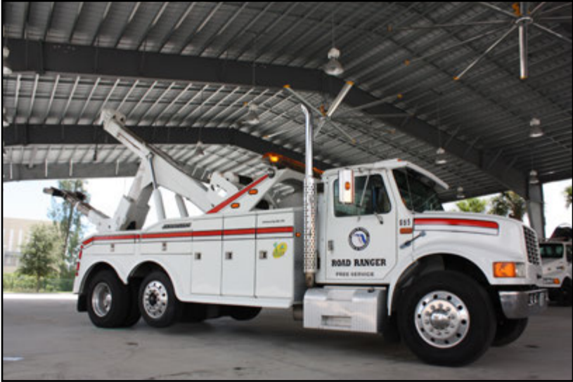
Heavy-duty wrecker truck to expedite clearance or road-blocking incidents.
