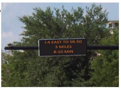
The DMSs are National Transportation Communications for ITS Protocol compliant, which allows integration into the SunGuide<sup>TM</sup> software system. FDOT District 5 can communicate with the DMS and automatically display travel time information based on input from transponder readers on I-4 and major arterials. The transponder readers were installed as part of the iFlorida project in 2006.
