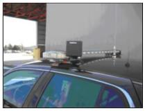
Additionally, MnPass is unlike the others as it does not utilize video enforcement, but relies on highway patrol and use of various other technologies to identify violators. One such technology is the use of a patrol vehicle mounted transponder reader/antenna which can interrogate passing vehicles and obtain recent MnPass lane transaction activity.
