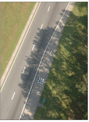
exit numbers and locations, directional guidance, and detours. In addition, this signage lessens the need for locating variable message signs along a contraflow route to provide the same highway information.
