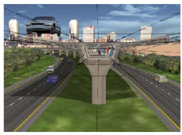
ITS components of the Reversible Express Lane Project will also provide an "open air" laboratory for testing new concepts in highway safety and a prototype for 21st century transportation facilities. The Reversible Express Lane Project includes a bridge design with a useable hollow core that will provide an ideal environment for locating utilities, fiber optics, and specialized equipment to improve safety and traffic flow.
