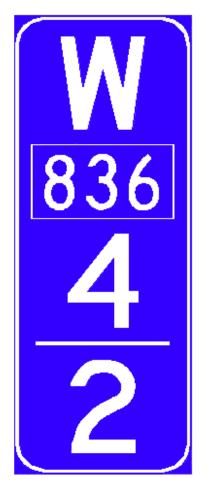
These markers are used in place of the standard milepost marker system and are typically placed at 0.1 or 0.2 mile intervals. The marker panels have white letters on a blue background, a nominal size of 18"x48", and provide the following information in a vertical format:
