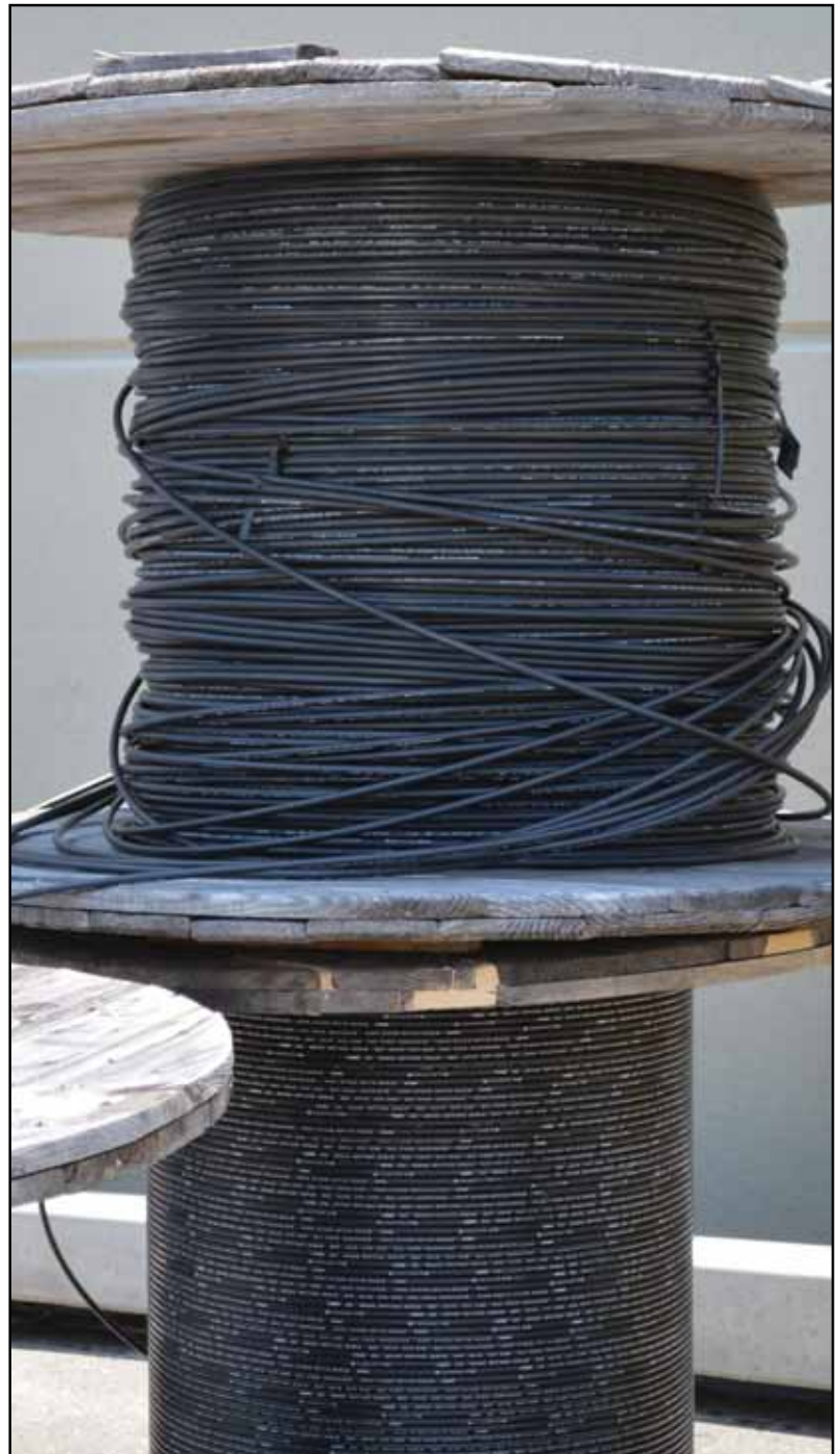
New and recycled fiber optic cable. Courtesy of FDOT District Seven
