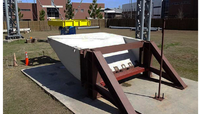
The replica barge is ready for experimental testing. The yellow and blue object just beyond the replica is the impact pendulum in its rest position.
