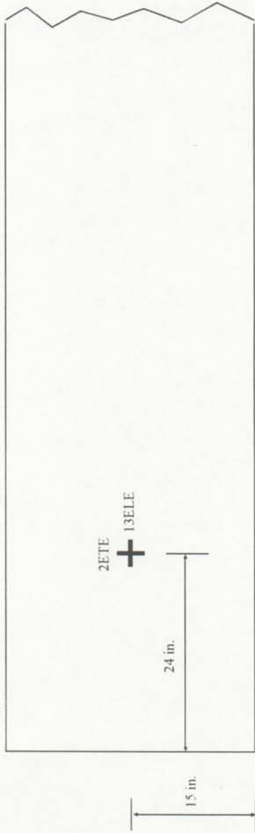
Pile 1 East Compression Face
