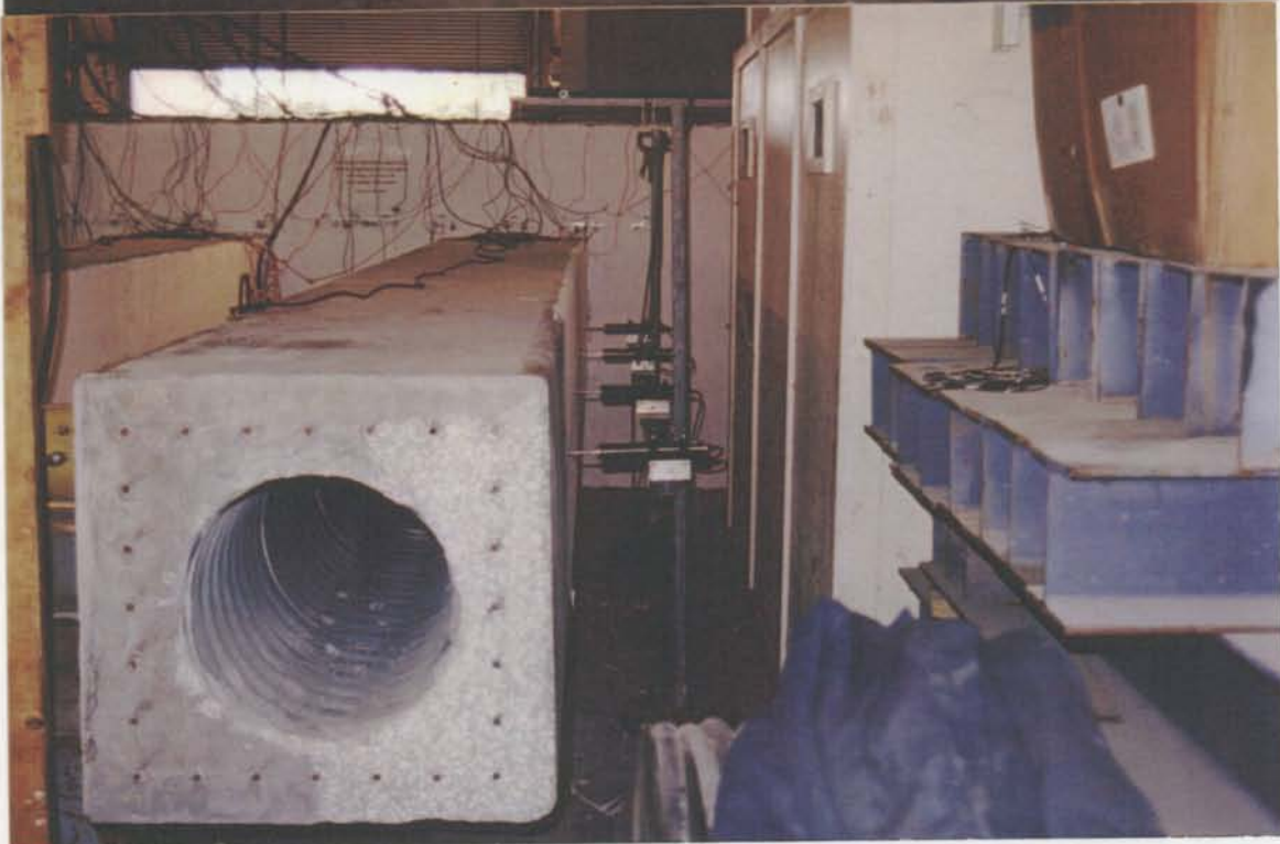
-Test Setup of the Test Specimen. -Installation of the LVDT's to Measure deflections along the Test Specimen.
