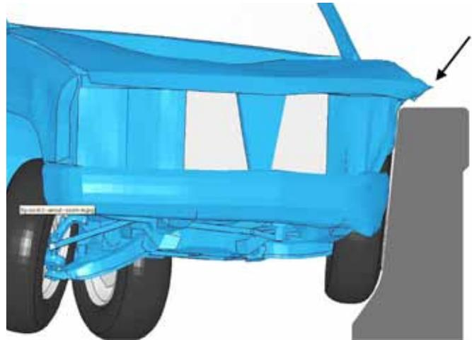
*This image from the simulation shows the model truck during impact with the traffic railing. The arrow shows the Zone of Intrusion, the region beyond the plane of the traffic railing into which the impact-deformed vehicle intrudes. The profile of the traffic railing is characteristic of the F-shape barrier.*
