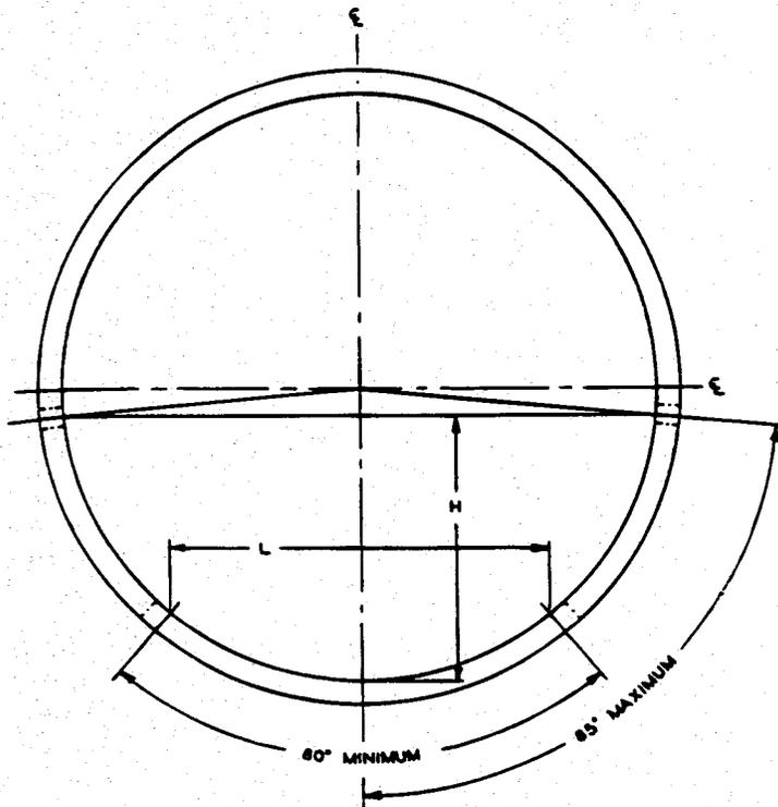
FIGURE 1 Circumferential Location of Class 1 Perforations
