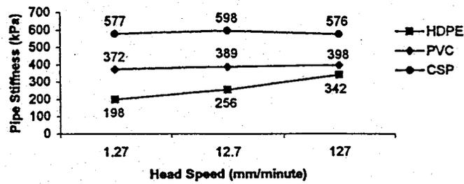
Figure A3.3 – Change in PS with strain rate (head speed) (600 mm pipes)
