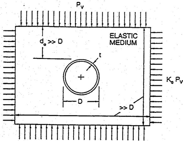
FIGURE 3 Burns and Richard model for pipe embedded in an elastic plate.
