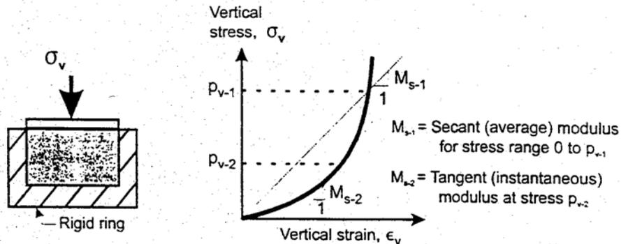
FIGURE 2 One-dimensional test and secant constrained modulus.
