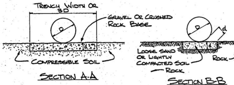
$d = \frac{1}{2}$  in./ft [40 mm/m] of fill over pipe, with a 24-in. [600-mm] maximum.
