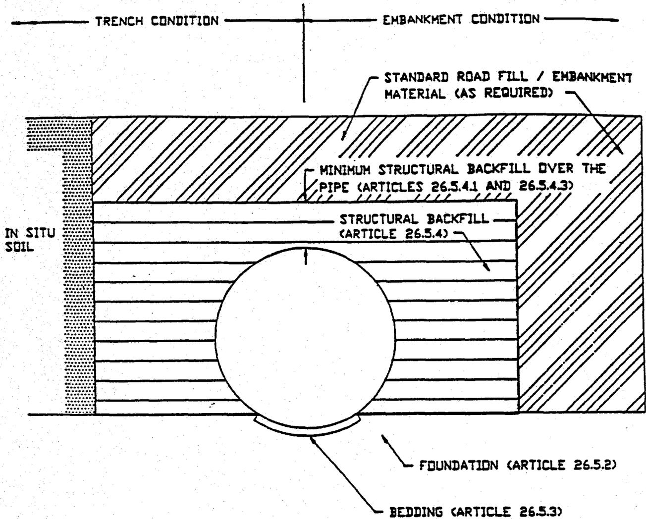
FIGURE 26.5 Typical Cross-Section Showing Materials Around the Pipe
