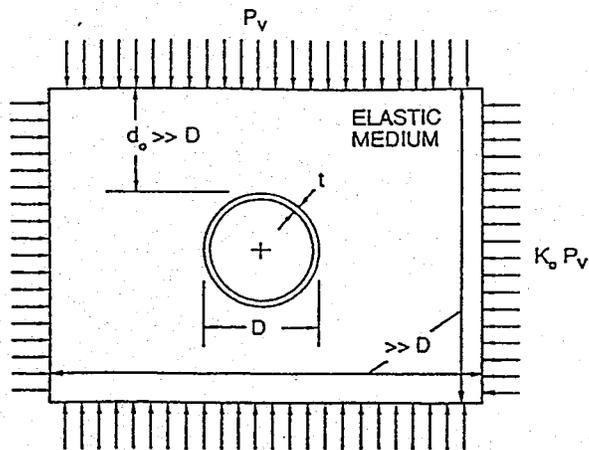
Figure A4.1 – Burns and Richard model for pipe embedded in an elastic plate.
