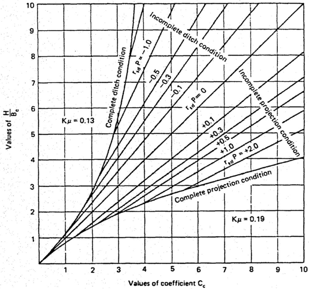
**Figure 3.4 – Diagram for coefficient  $C_c$  for positive projection pipes**
