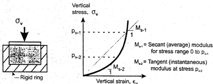
FIGURE 2 One-dimensional test and secant constrained modulus.
