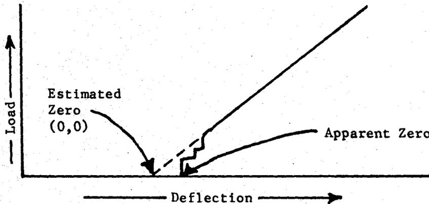
FIG. A1.1 Method of Estimating the Origin
