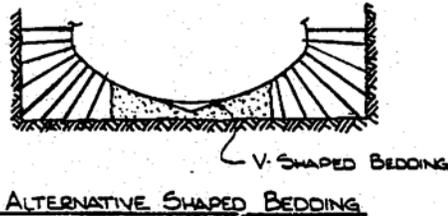
FIG. 3 Pipe Arch Bedding and Corner Zone Treatment—Ordinary Conditions
