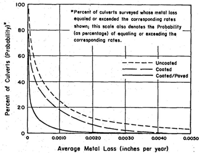
Figure A6.1 – Distribution of average metal loss for galvanized steel culverts (after Haviland, Bellair, and Morrell, 1967).
