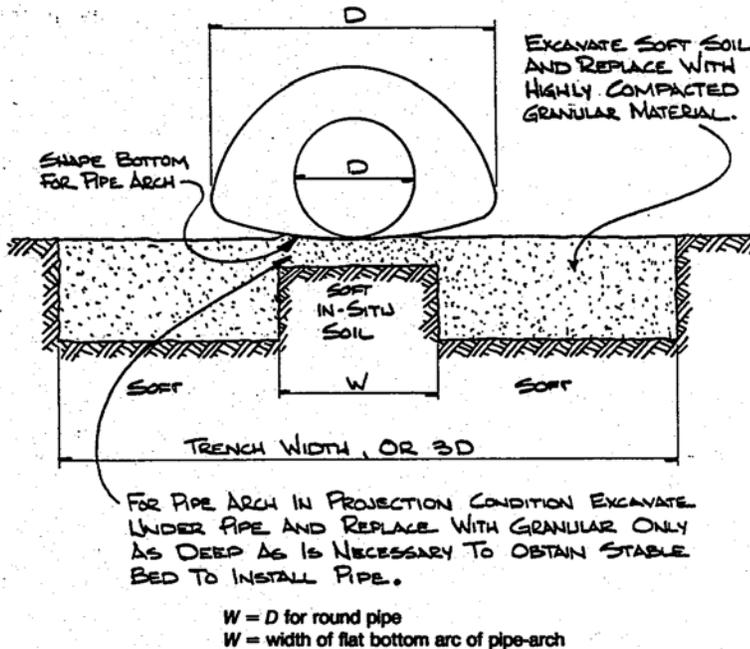
FOR PIPE ARCH IN PROJECTION CONDITION EXCAVATE UNDER PIPE AND REPLACE WITH GRANULAR ONLY AS DEEP AS IS NECESSARY TO OBTAIN STABLE BED TO INSTALL PIPE.
