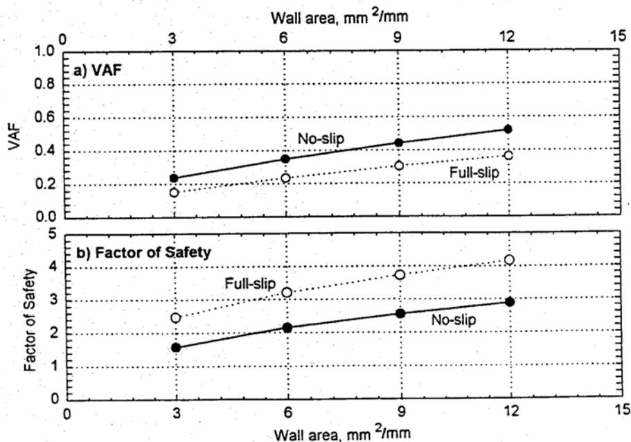
FIGURE 7 Effect of changing wall area on VAF and factor of safety.
