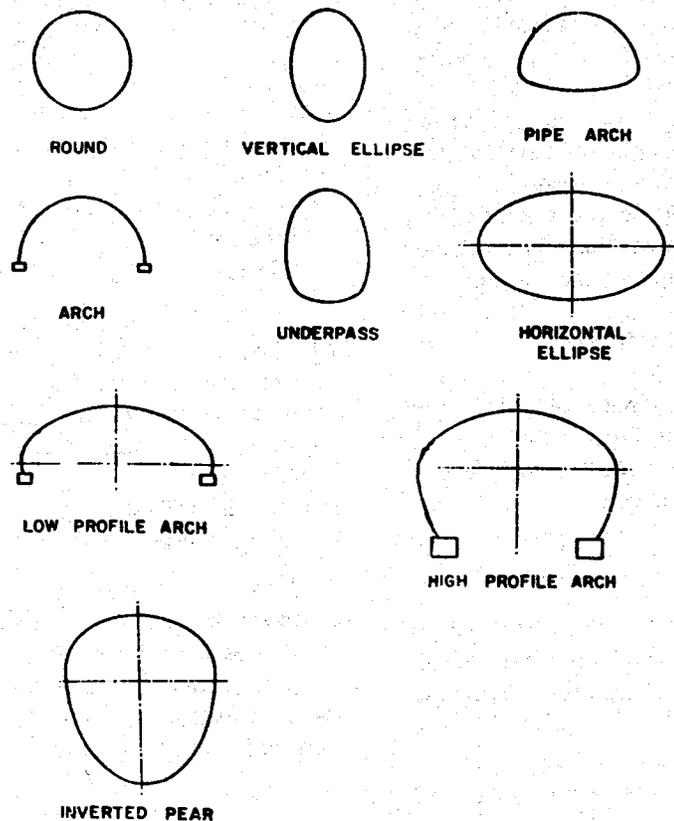
Figure 12.7.1A. Standard Terminology of Structural Plate Shapes Including Long-Span Structures
