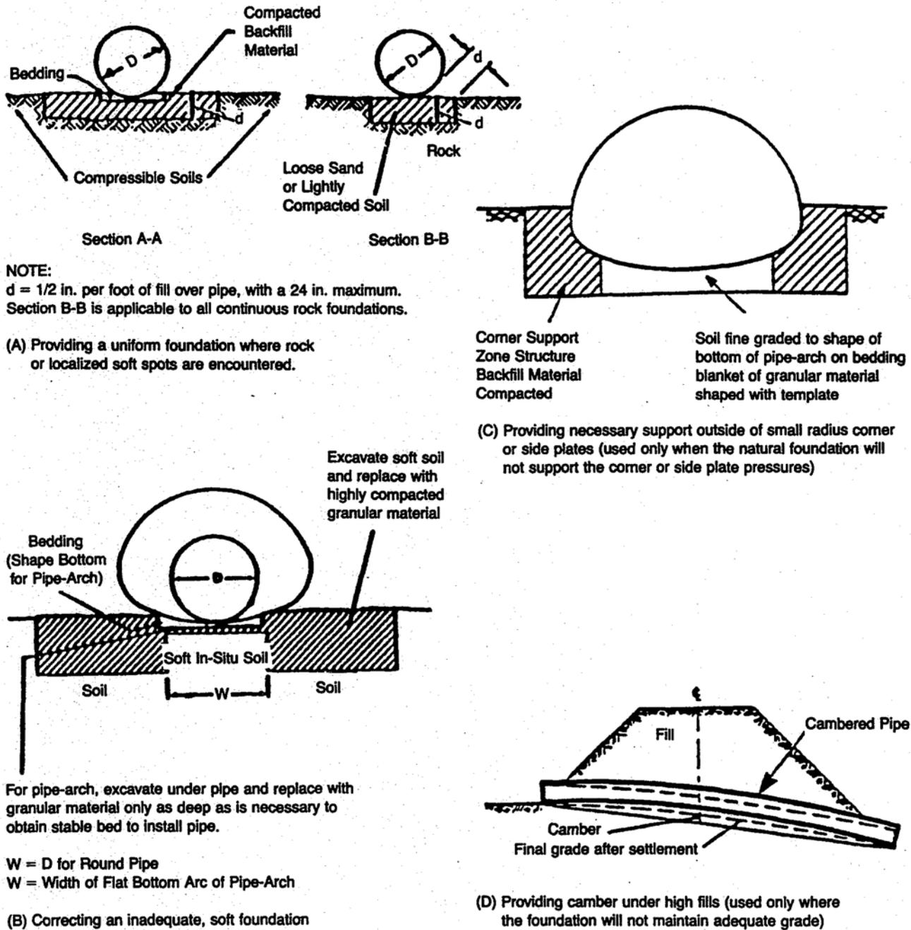
FIGURE 26.5.2 A-D: Foundation Improvement Methods when Required
