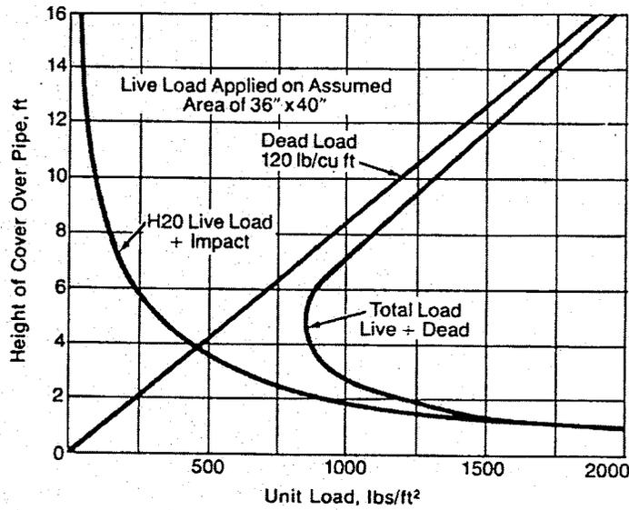
(a) Combined HS20 highway live load and dead load is a minimum at about 5 ft cover, applied, through a pavement 1 ft thick
