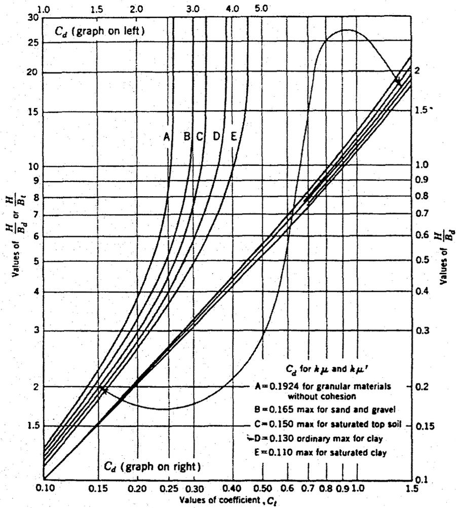
**Figure 3.2 – Computation diagram for earth loads on trench conduits completely buried in trenches (Source : Moser, 1990)**
