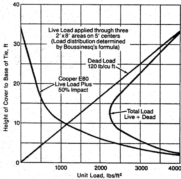
(b) Railroad live load, Cooper E80, combined with dead load is a minimum at about 12 ft. Load is applied through three  $2 \times 8$  ft areas on 5 ft centers.
