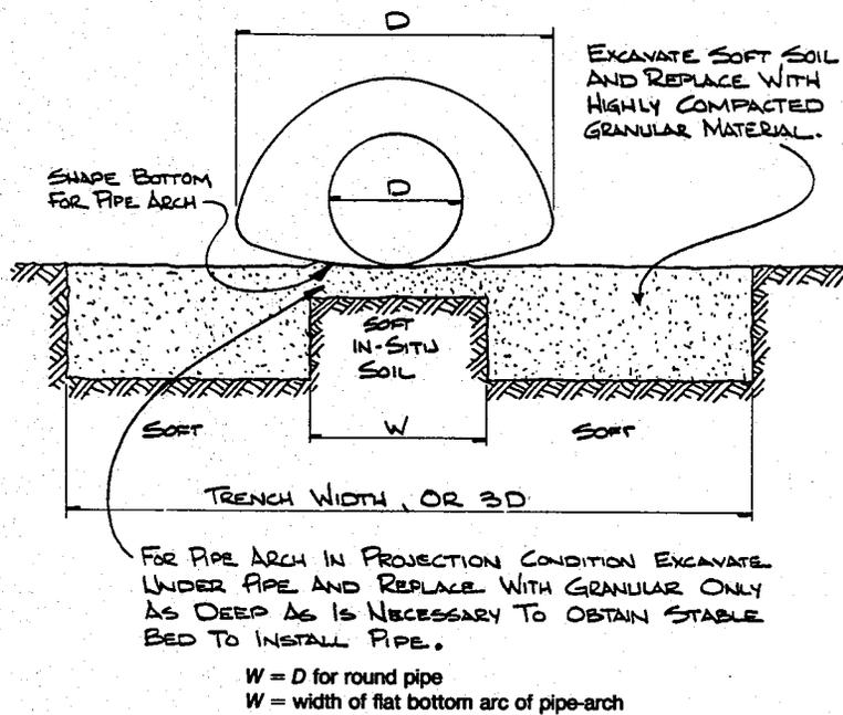
FIG. 5 Soft Foundation Treatment for Larger Pipe and Pipe-Arch
