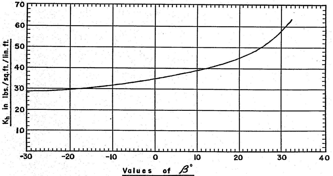
Figure C12.6.2.2.5-2 - Lateral Earth Pressure as a Function of Ground Slope
