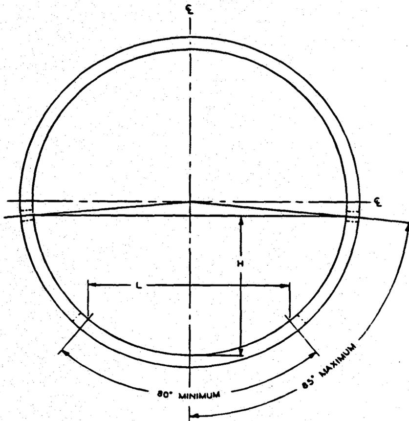
FIGURE 1 Requirements for Perforations
