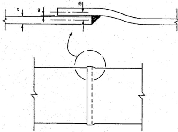
**Figure A5.1 – Bell-and-Spigot Joint**
