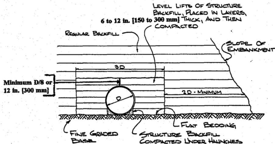
FIG. 2 Ordinary Embankment Condition
