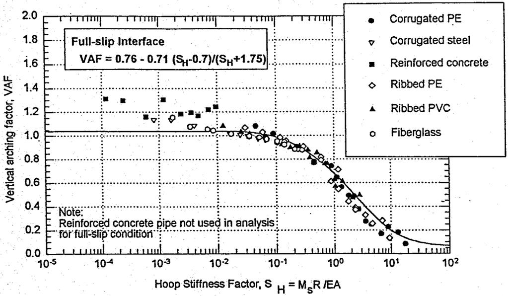
Figure A4.3 – Burns and Richard VAF : full-slip interface. PE = polyethylene;
