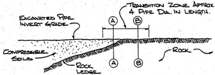
TRANSITIONS OF PIPE FOUNDATIONS FROM COMPRESSIBLE SOILS TO ROCK. EXCAVATE ROCK AND COMPRESSIBLE SOIL IN TRANSITION SECTION TO PROVIDE REASONABLY UNIFORM LONGITUDINAL PIPE SUPPORT AND MINIMUM DIFFERENTIAL SETTLEMENT.
