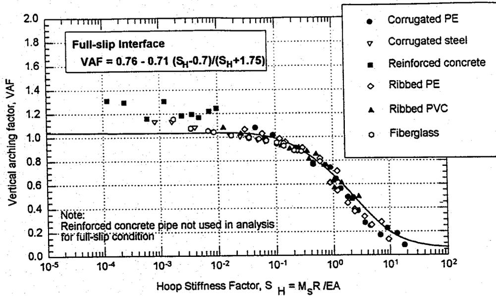
FIGURE 5 Burns and Richard VAF: full-slip interface. PE = polyethylene; PVC = polyvinyl chloride.
