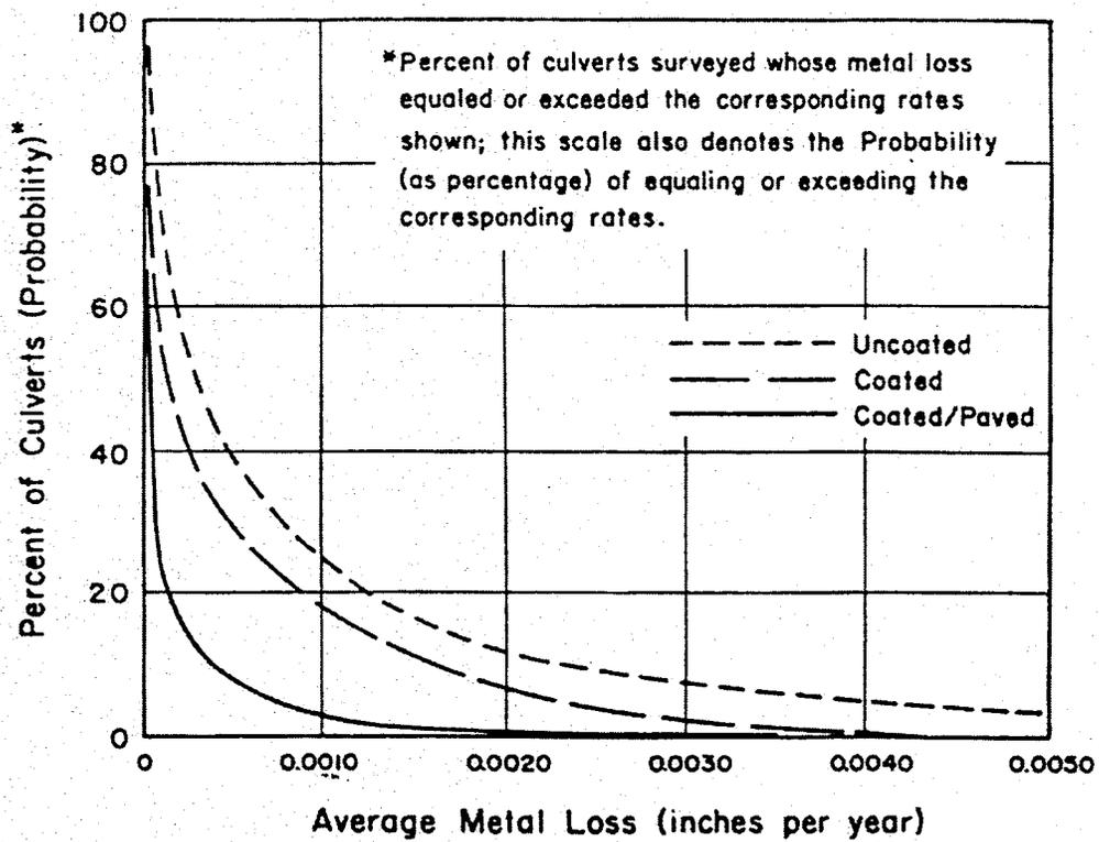
**Figure 3.8 – Distribution of average metal loss for galvanized steel culverts**
