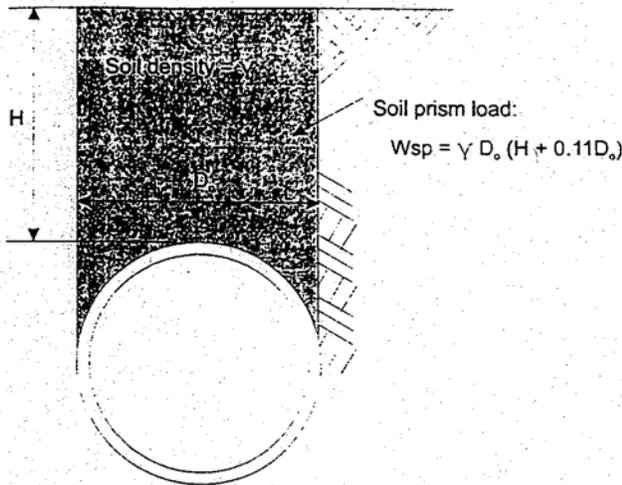
FIGURE 1 Definition of soil prism load.
