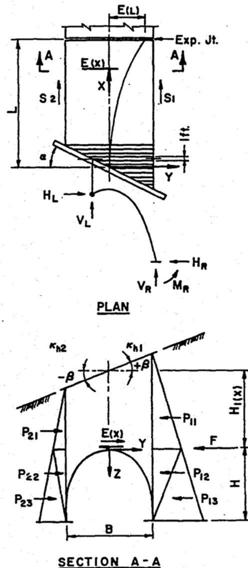
Figure C12.6.2.2.5-1 - Forces on Culvert - Approximate Analysis
