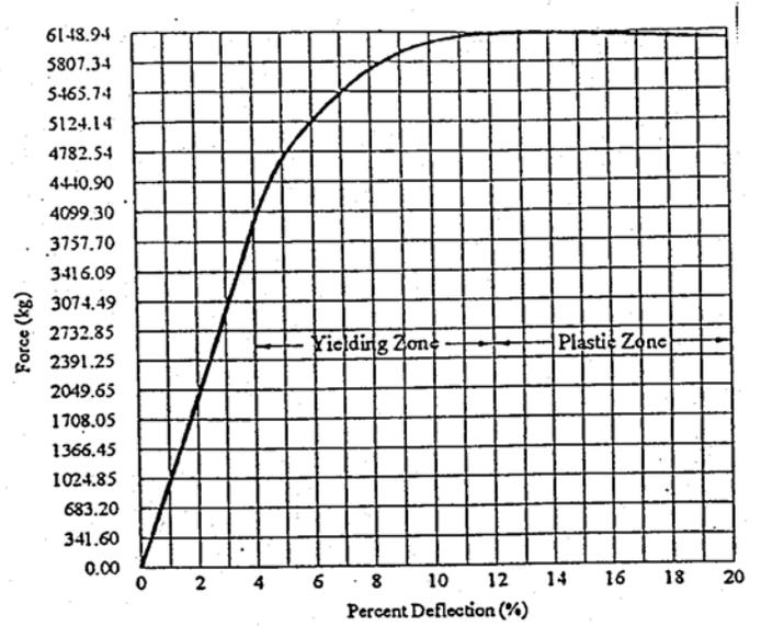
Figure A3.2 – Load-deflection curve (450 mm CSP)
