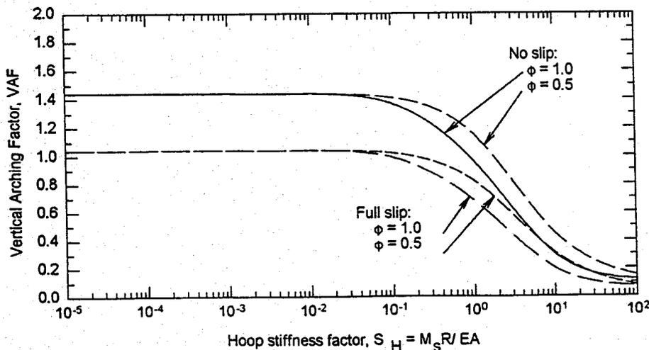
FIGURE 6 Sensitivity of VAF to variations in soil stiffness.
