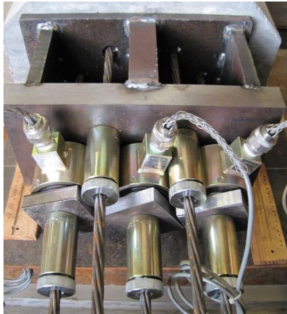
Figure 52–Detensioning chair, chucks, and load cells on the unbonded segment
