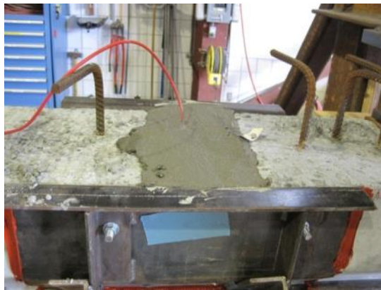
Figure 59–Top of finished closure pour
