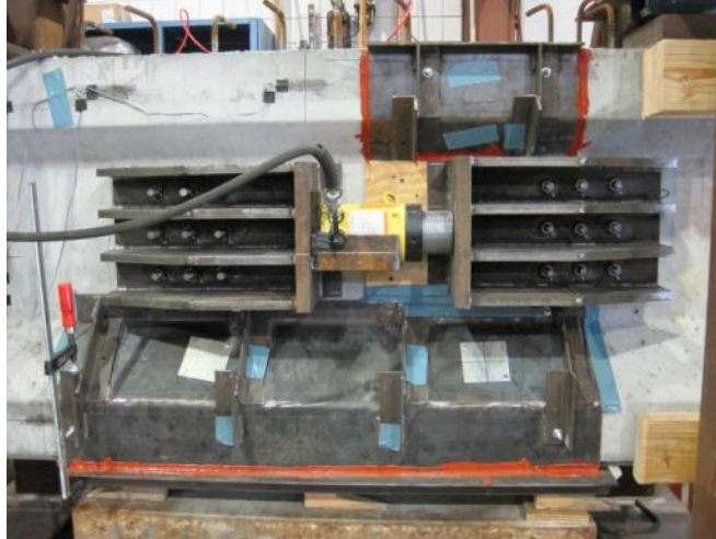
Figure 56–Closure formwork in place
