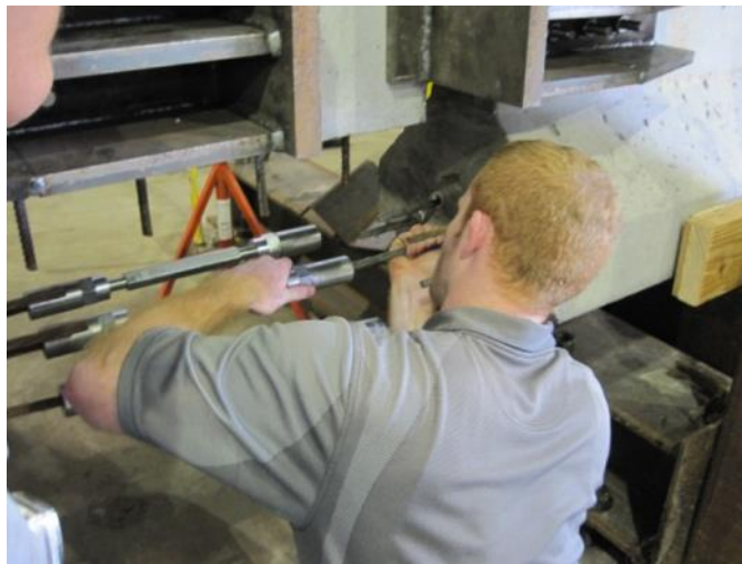
Figure 48–Coupler installation on unbonded strand
