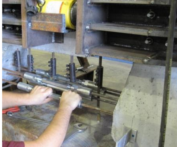
Figure 53–Tightening the turnbuckles to seat detensioning chair
