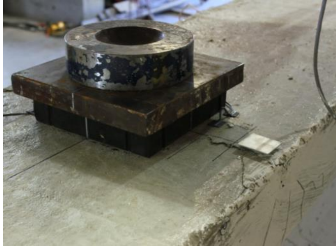
Figure 122–SB: Deck at failure
