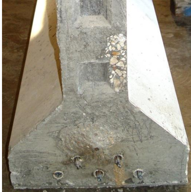
Figure 142–Post-test: End view of unbonded segment
