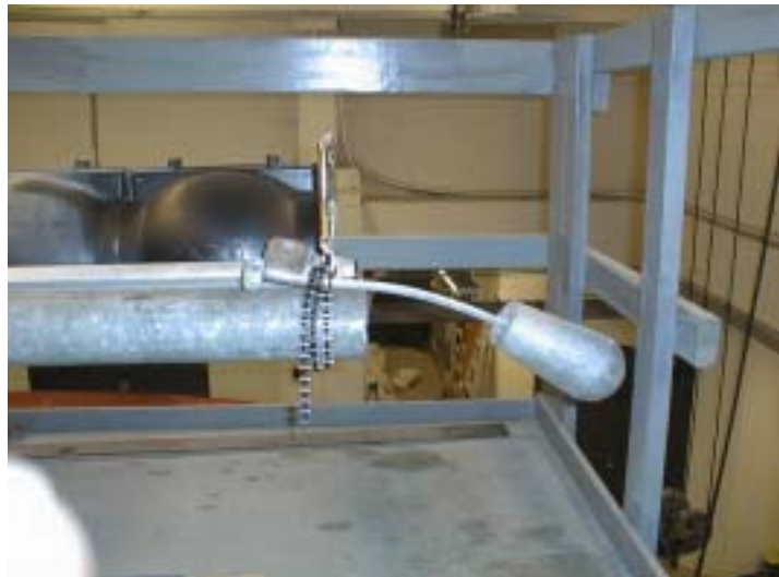
Figure 3.10 - Stockbridge Version Damper
