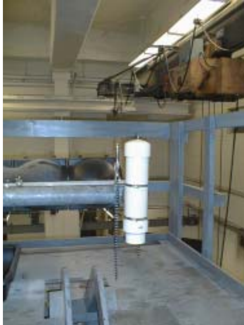
Figure 3.33 - 4 in to 3 in Tapered Spring/Mass Impact Damper
