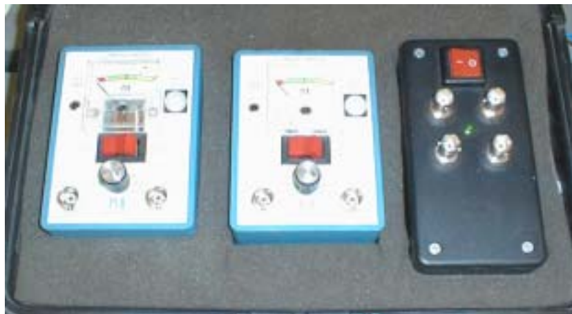
Figure 4.4 - Accelerometer Power Supplies and Filter
