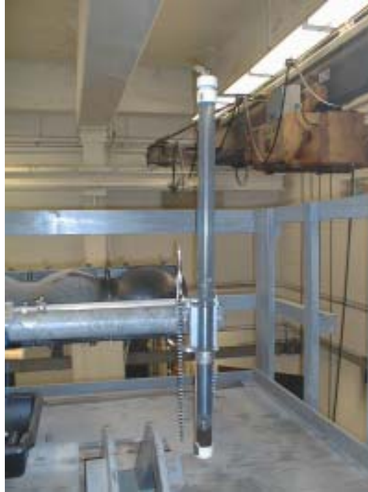
Figure 3.23 - 2 in PVC Pipe, Bungee and Mass Damper with Oil
