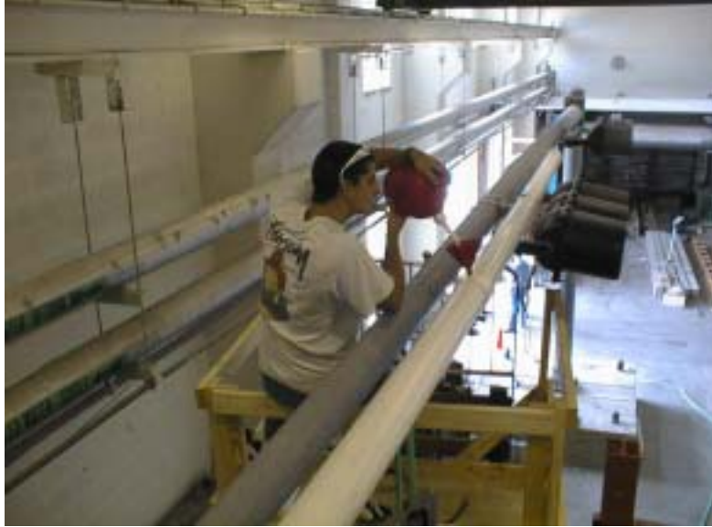
Figure 3.13 - 20 ft Long PVC Liquid Damper
