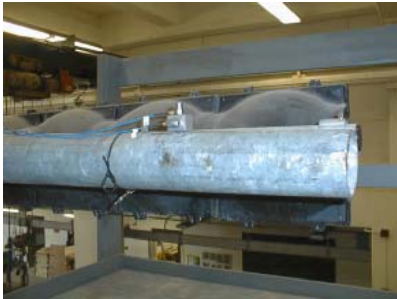
Figure 4.3 - Accelerometers attached to tip of lab mast arm
