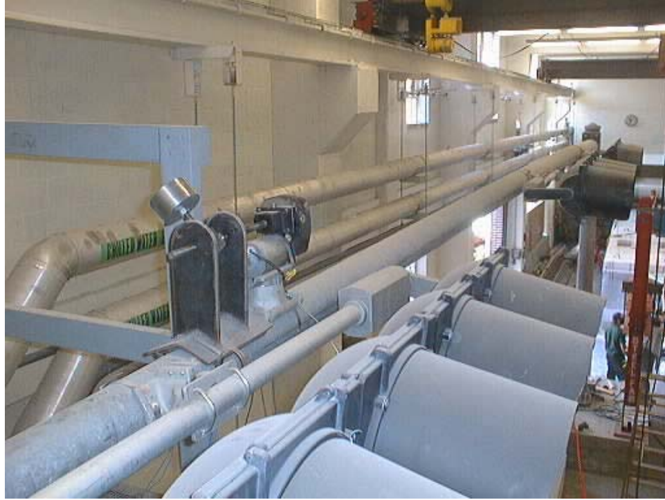
Figures 5.7 - Eccentric Mass and Motor Device (Photo 1)
