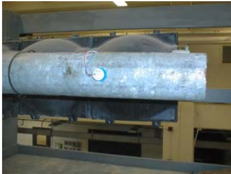
Figure 4.2 - Inclinometer attached to tip of lab mast arm
