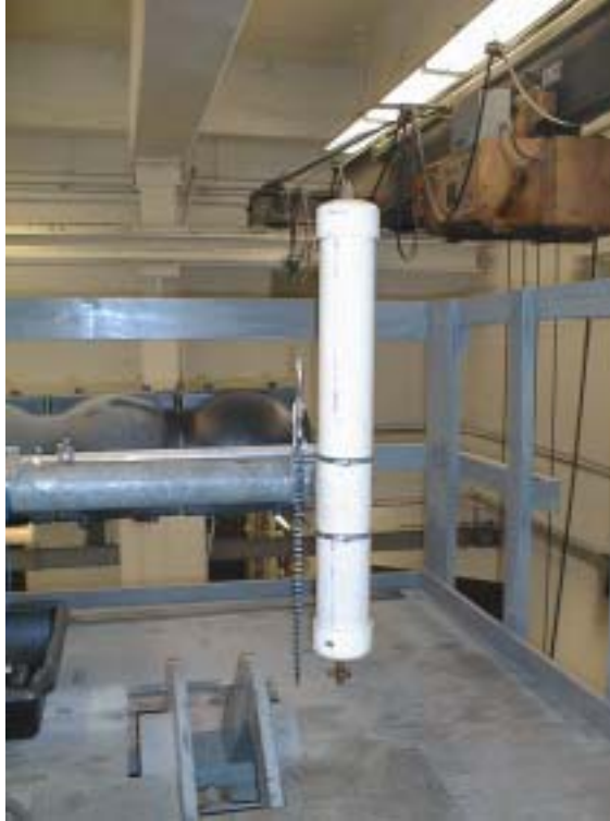
Figure 3.25 - 4 in PVC Pipe, Spring and Mass Damper with Oil
