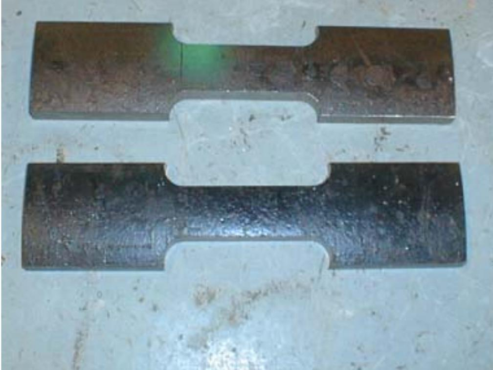
Figure 4.1 Coupons for pipe tensile strength tests
