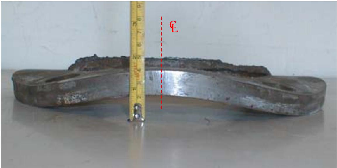
Figure 5.7 Deformation in tension region of Specimen #2
