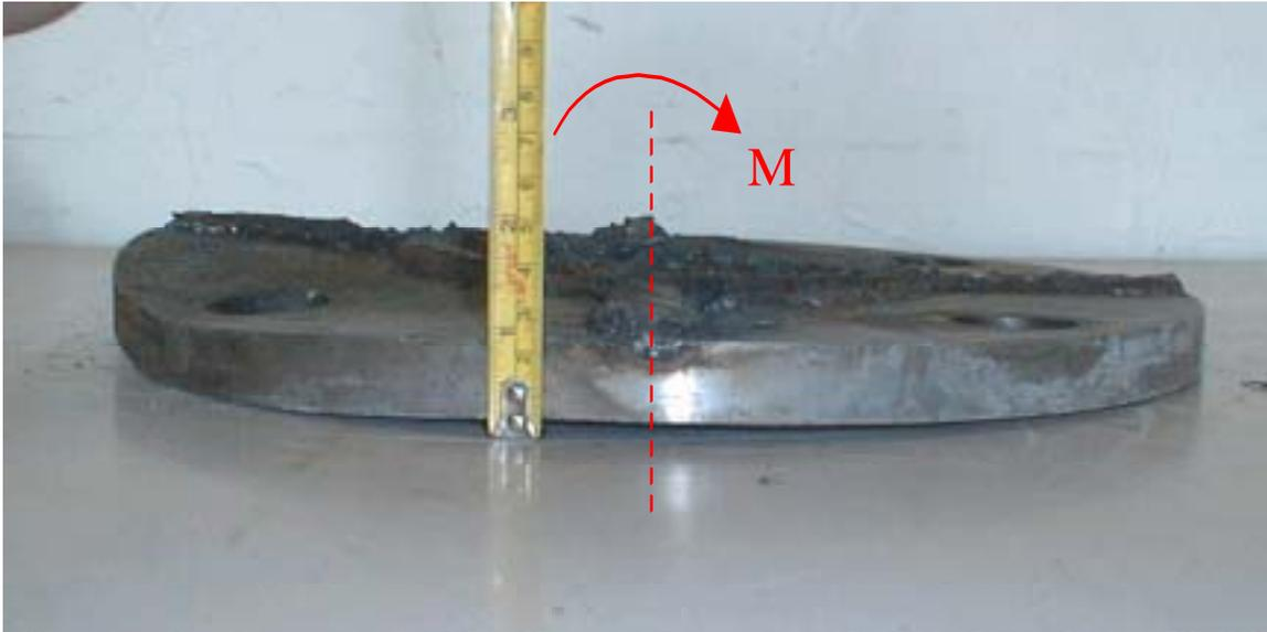
Figure 5.9 Deformed shape at axis of bending of Specimen #3
