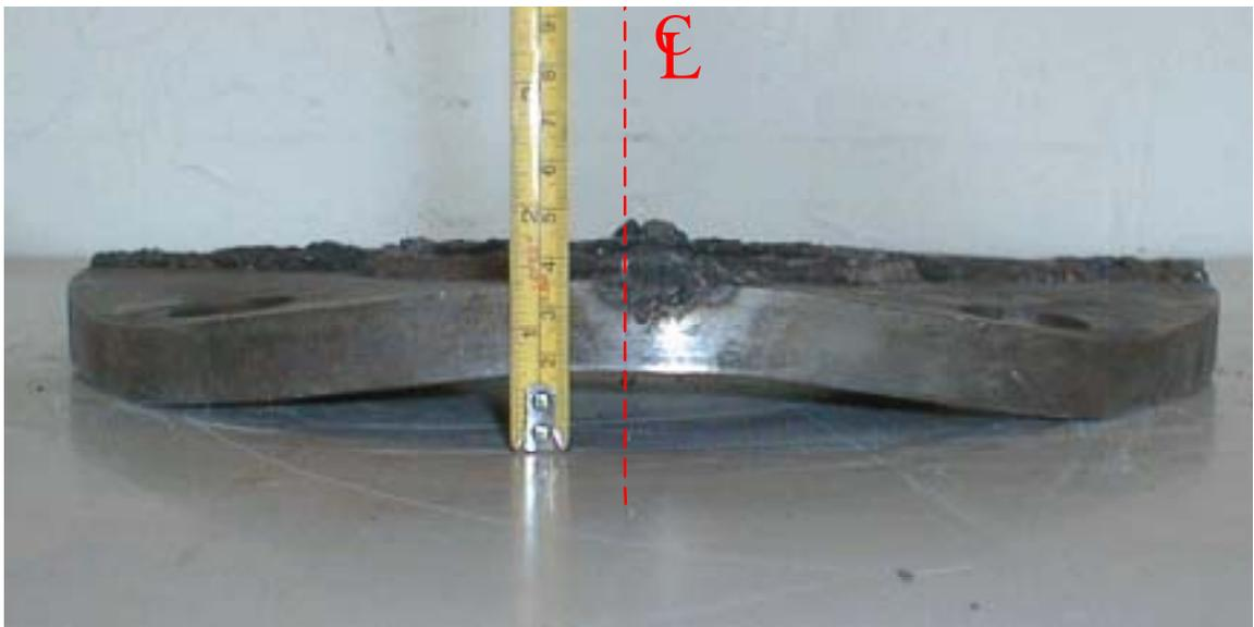
Figure 5.13 Deformed shape in tension region of Specimen #4
