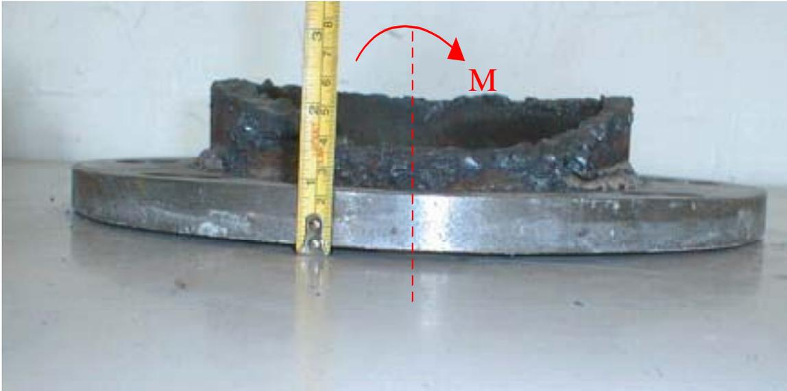
Figure 5.2 Deformed shape in tension region of Specimen #1
