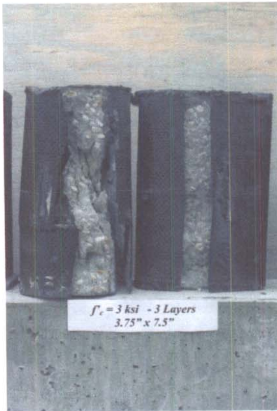
Fig. 4.3 a) - Typical Failure of Specimens ( a/b=0.50 ), Series 3: 3 ksi Concrete
