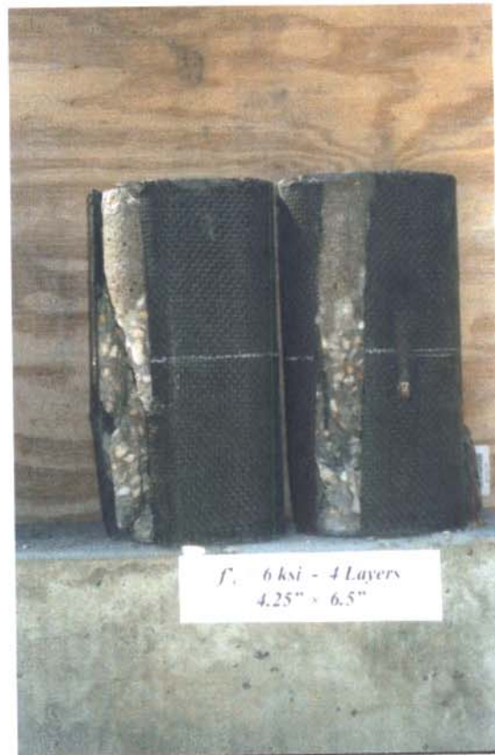
Fig. 4.2 b) - Typical Failure of Specimens ( a/b=0.65 ), Series 5: 6 ksi Concrete
