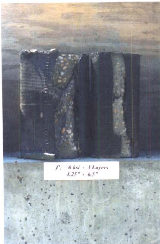
Fig. 4.2 b) - Typical Failure of Specimens ( a/b=0.65 ), Series 5: 6 ksi Concrete
