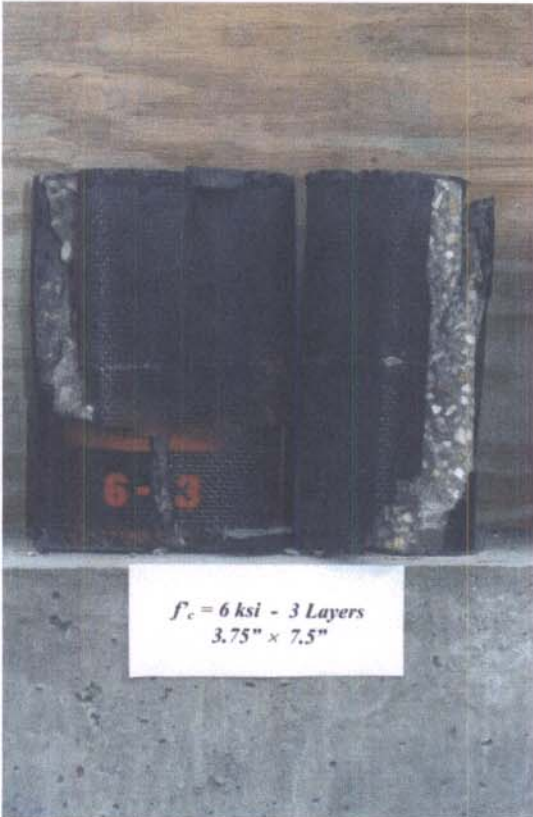
Fig. 4.3 b) - Typical Failure of Specimens (alb=0.50), Series 6: 6 ksi Concrete
