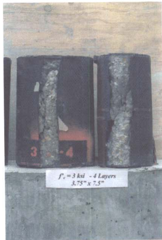
Fig. 4.3 a) - Typical Failure of Specimens ( a/b=0.50 ), Series 3: 3 ksi Concrete
