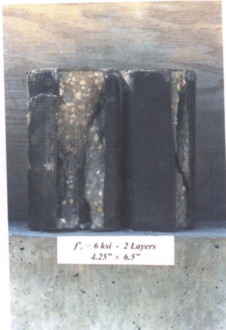
Fig. 4.4 - Typical View of Inside Wrapped Specimen After Test
