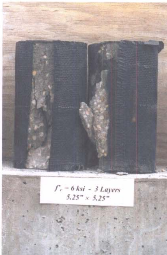
Fig. 4.1 b) - Typical Failure of Specimens (alb=1), Series 4: 6 ksi Concrete
