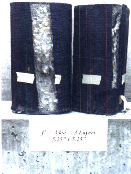
Fig. 4.1 a) - Typical Failure of Specimens (a/b=1), Series 1: 3 ksi Concrete
