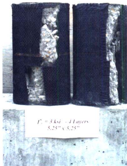
Fig. 4.1 a) - Typical Failure of Specimens (a/b=1), Series 1: 3 ksi Concrete
