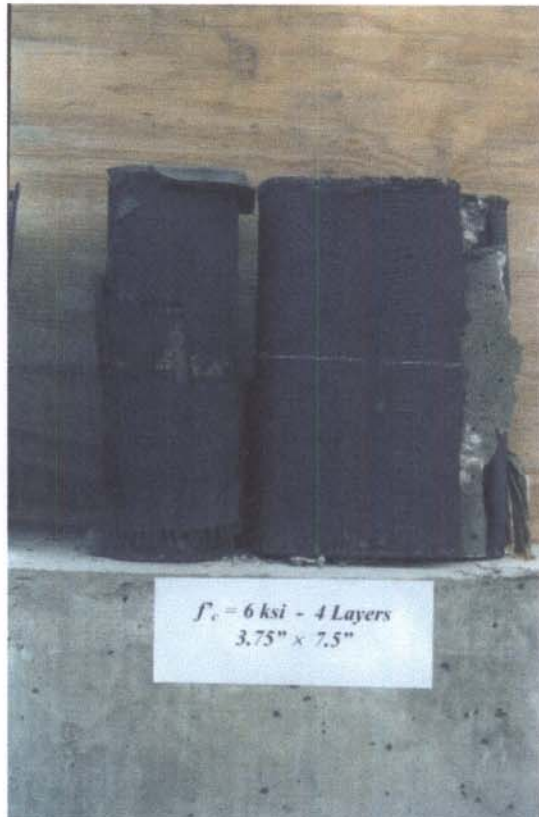
Fig. 4.3 b) - Typical Failure of Specimens (alb=0.50), Series 6: 6 ksi Concrete
