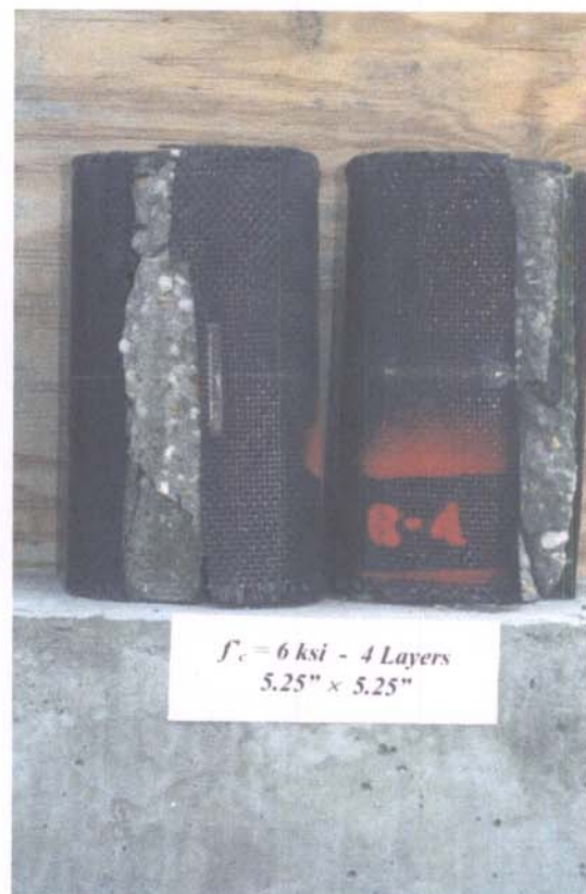
Fig. 4.1 b) - Typical Failure of Specimens (alb=1), Series 4: 6 ksi Concrete
