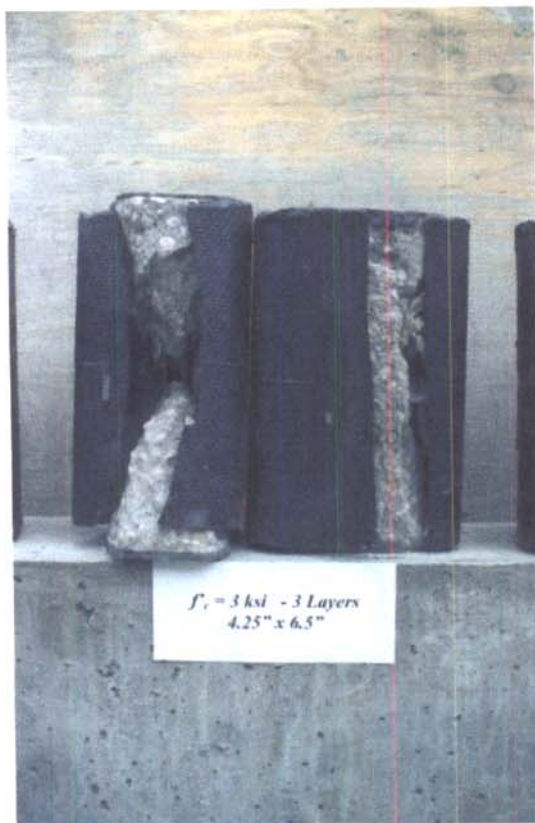
Fig. 4.2 a) - Typical Failure of Specimens ( \alpha_b=0.65 ), Series 2: 3 ksi Concrete
