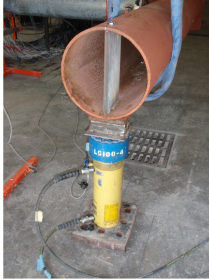
Figure 4-10. Load cell and actuator used for applying load to test apparatus. Photo courtesy of S. Dalton.
