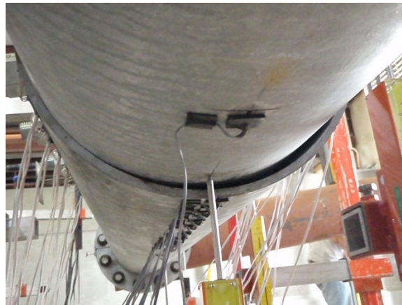
Figure 5-11. Oblong deformation at the base of the outer pole during loading. Photo courtesy of S. Dalton.
