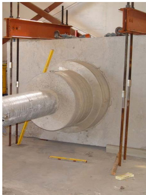
Figure 3-9. Tie-down assemblies connecting the base of the test apparatus to the lab floor. Photo courtesy of FDOT.
