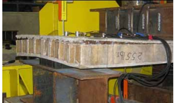
A section of GFRP deck is loaded to failure in a laboratory setup.
