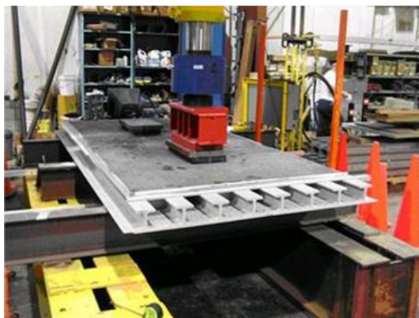
Figure 105 – Structural test of GFRP deck used in Belle Glade bridge (Vyas et al. [2009])
