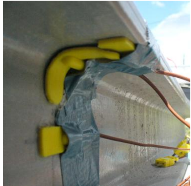
Figure 27 – Surface-temperature-measuring thermocouples on panel B8
