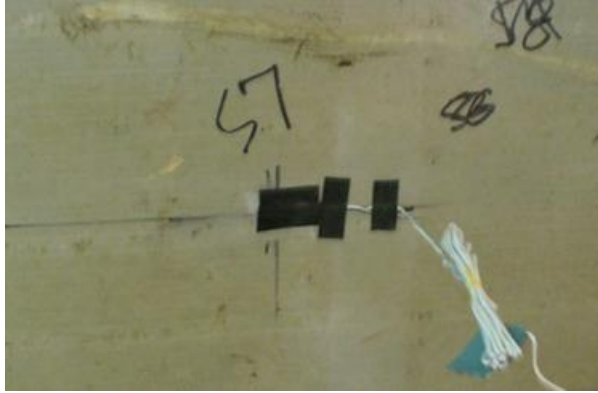
Figure 25 – Bonded strain gage
