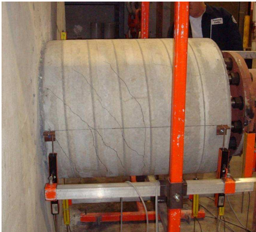
Figure 5-10. Formation of concrete breakout failure cracks in second test
