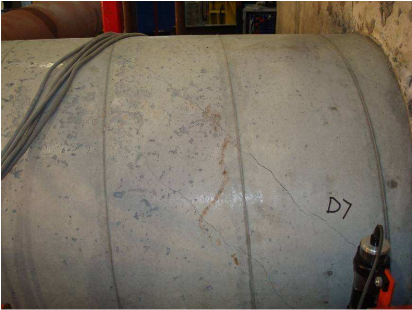
Figure 5-2. Formation of torsional cracks
