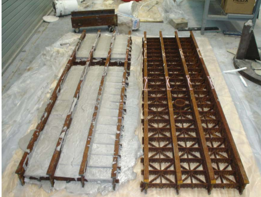
Figure 3-3: Pouring of E-Bond 526 LW Materials to Open Steel Grate Decks.
