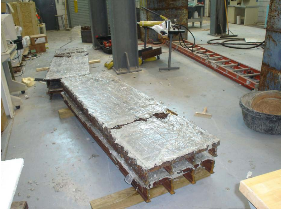
Figure 3-4: Filled Open Grate Deck with E-Bond 526 LW Materials.
