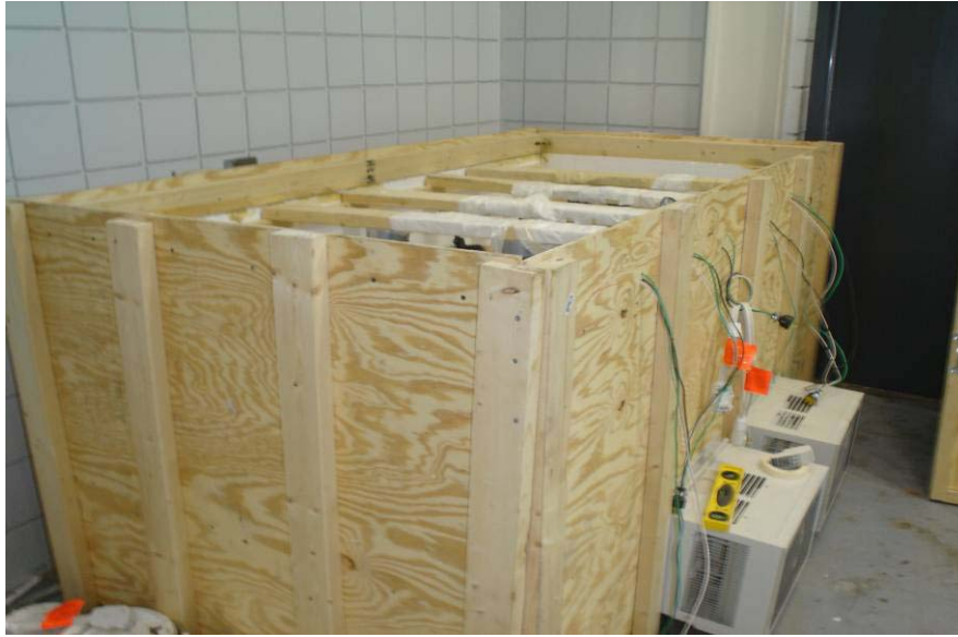
b) Climate Controlled Chamber Showing Cooling Units for Cool Zone
