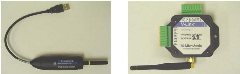
Figure A.4 – Microstrain data acquisition and transmitter
