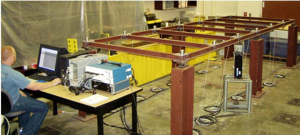
Figure B.12 – The physical grid model and test setup
