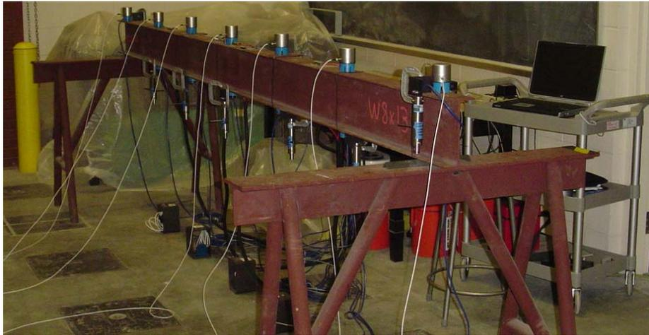
(a) Instrumented steel beam
