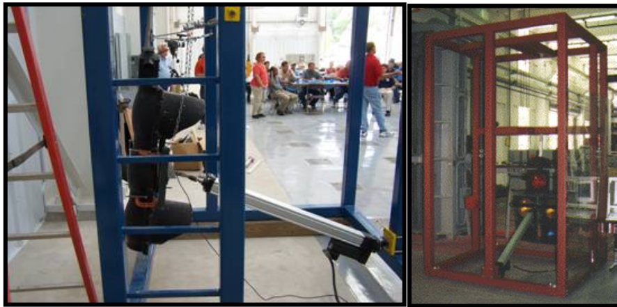
Figure 2-2. Test apparatus created for testing of traffic signal components.
