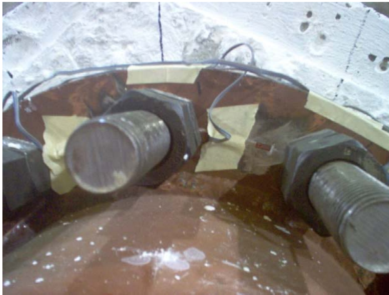
Figure 4-11. Strain gage on base plate of test specimen
