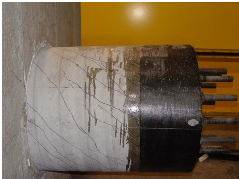
Figure 5-15. Torsion cracks along length of the shaft after the test
