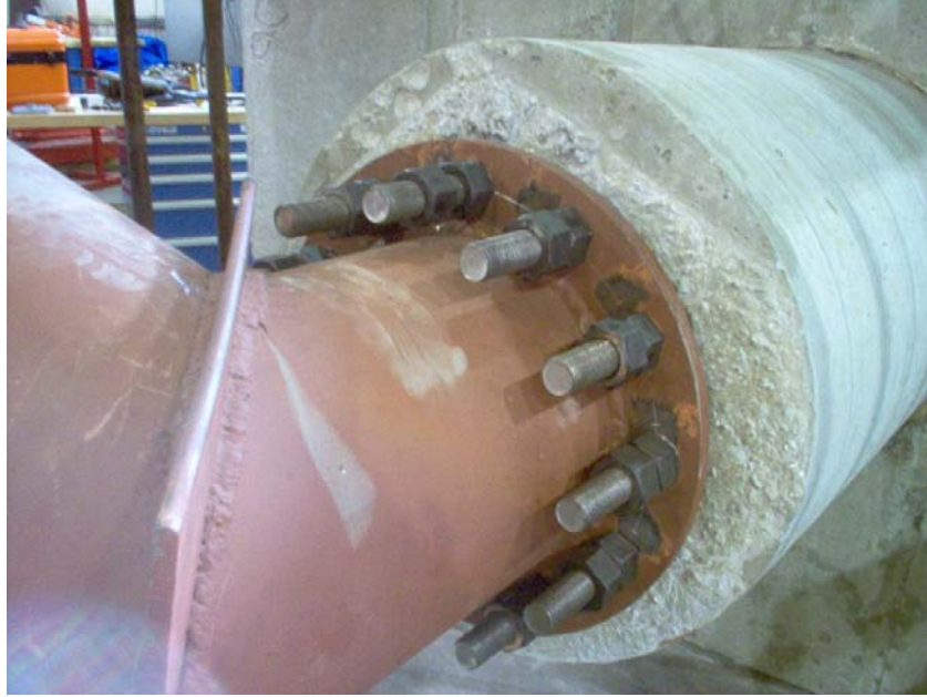
Figure 3-13. Shaft with pipe apparatus attached prior to instrumentation being attached
