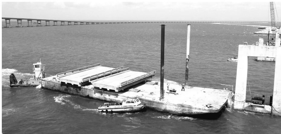
Figure 3.4 Test barge with payload impacting Pier-1 in the series P1 tests
