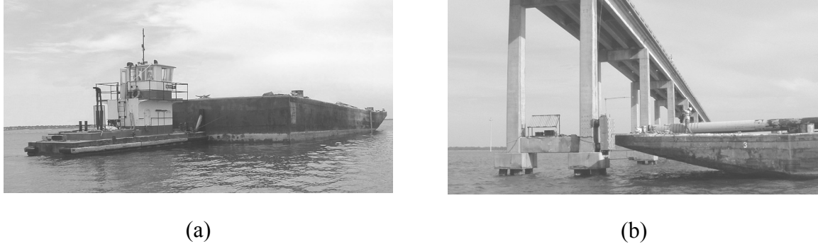
Figure 3.5 Series B3 tests: a) Empty test barge used in the series B3 tests, and b) Test barge impacting the bridge at Pier-3 during the series B3 tests
