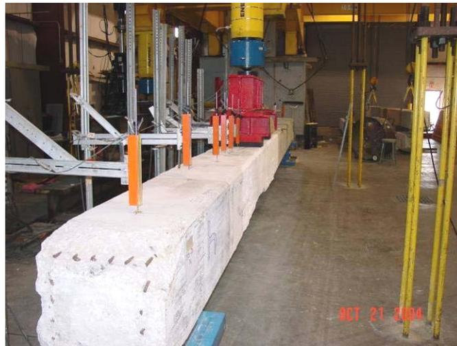
Figure 16 – Instrumentation for flexural testing
