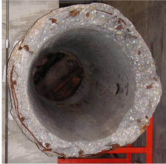
Figure 39 – Open end of pile
