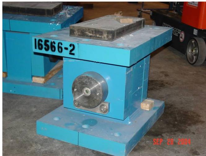
Figure 15 – Biaxial clevis load cell
