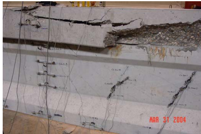
Figure 35. Failed F2-SCCF1 beam
