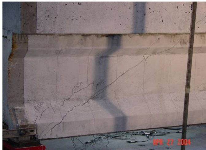
Figure 42. Failed SS2-SCCF2 beam
