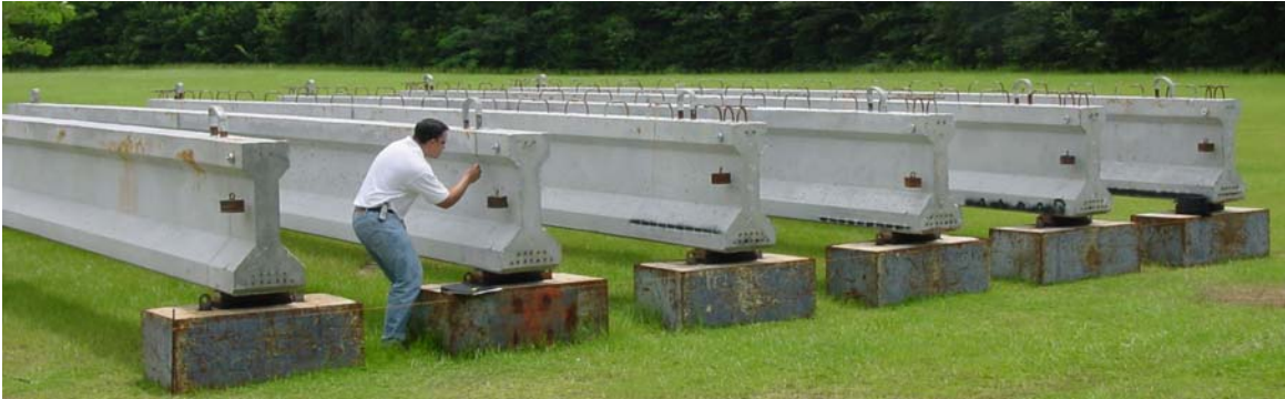
Figure 10. Camber monitoring of beams
