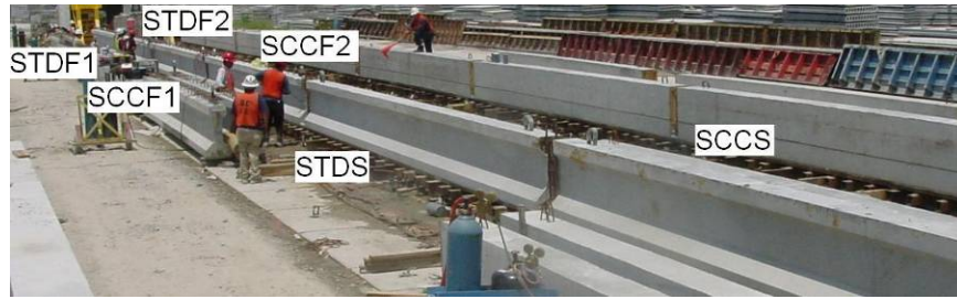
Figure 53. Specimen configuration in prestressing bed
