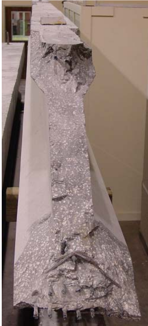
Figure 33. SCCS girder after shear testing. Note higher density of aggregate in the bottom of beam than in the top.
