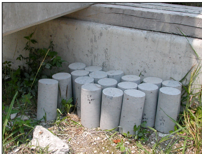
Figure 11. Field cured 4"x 8" concrete test cylinders.
