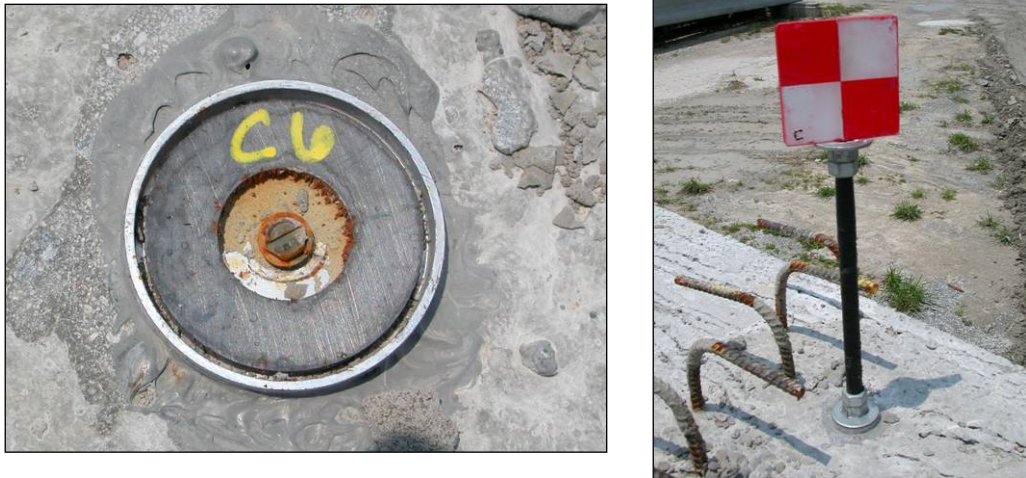
Figure 5. Optical target mounted on fixed ceramic magnet
