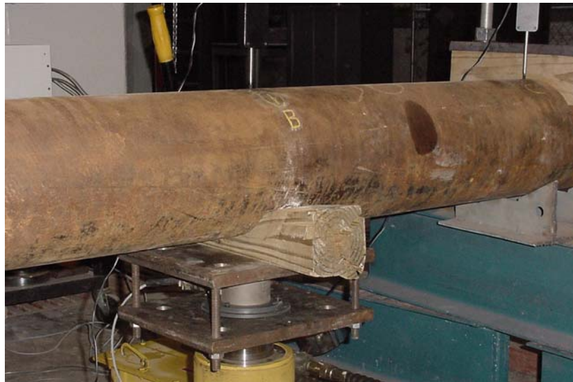
Figure 2.16 Laboratory Mini-Pile Test
