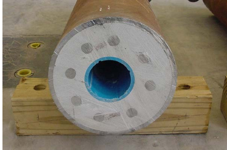
Figure 2.14 Five Foot Test section of Mini-pile
