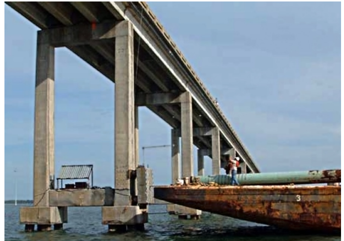
A moving barge strikes a bridge pier during a collision experiment.
