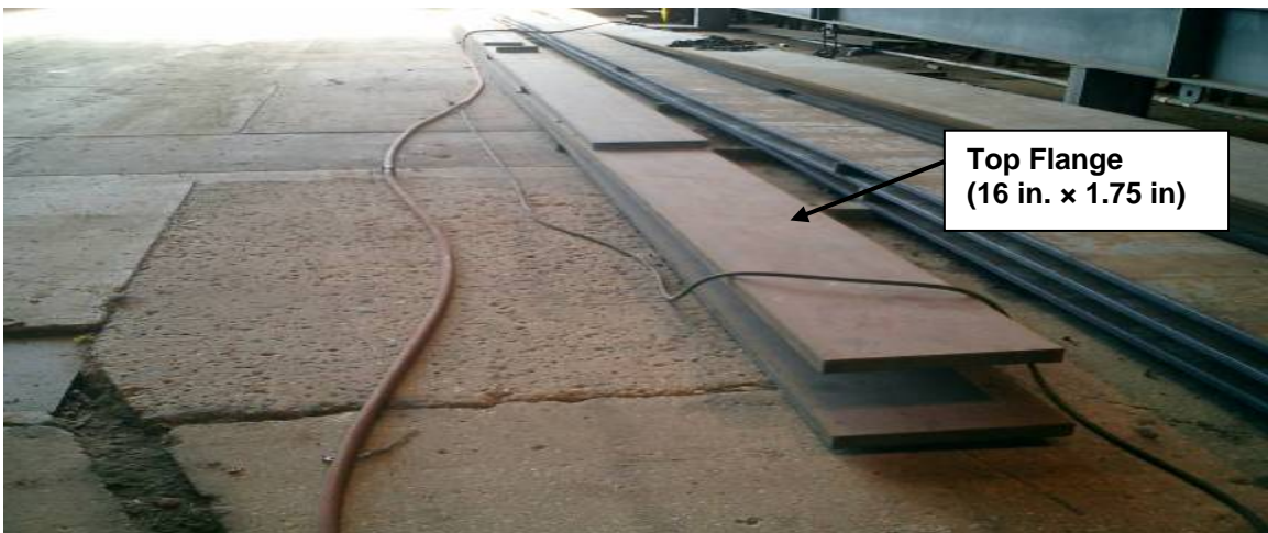
Figure 3.2 Cut Pieces from Plates
