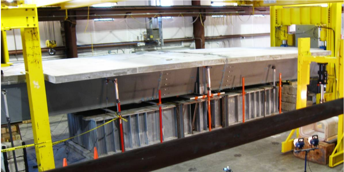
Figure 6.1 Deflected Shaped of Double Composite Box Girder
