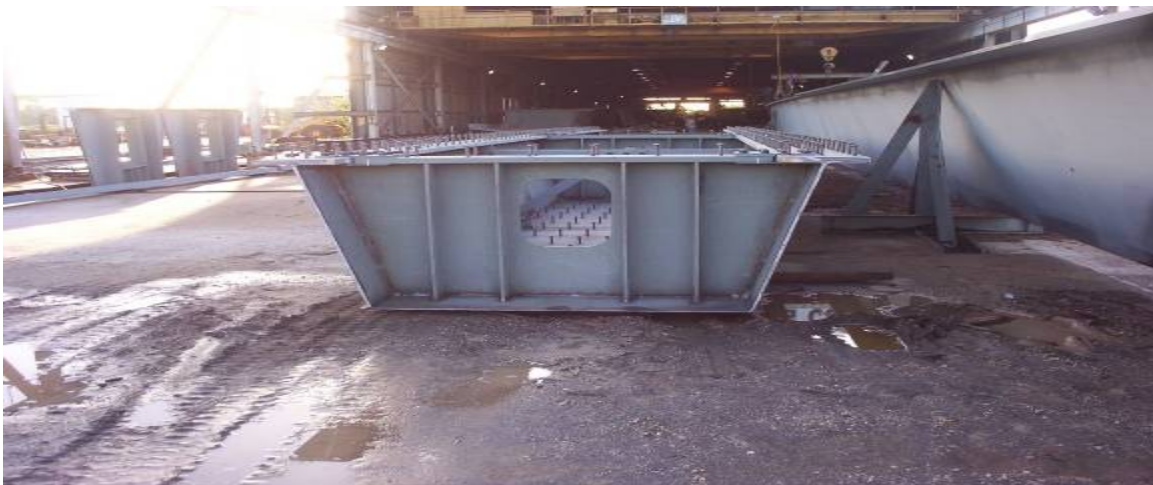
Figure 3.13 Steel Box Girder Ready for Shipment to Tallahassee
