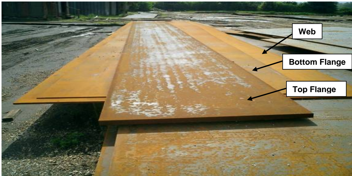
Figure 3.1 HPS Steel Plates from Mill
