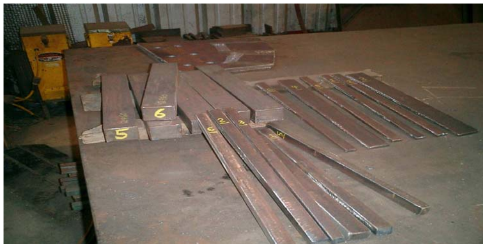
Figure B.1 Photograph of Coupon Test Specimens Tested at Gainesville – August 2008
