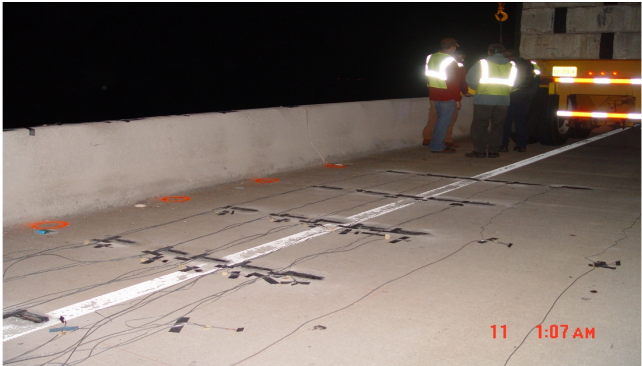
Figure 40: Truck Positioning for Channel Five Bridge Test.
