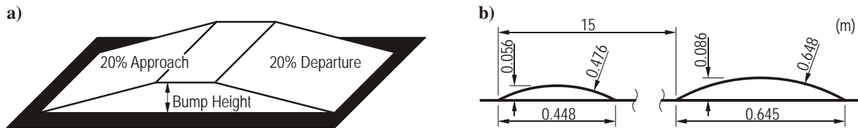
Figure 2.7. Different types of obstacles (bumps) used in the suspension tests for following vehicles: a) heavy 5-axle tactical military truck (Letherwood & Gunter, 2001), b) agricultural tractor (Lehtonen, 2005)
