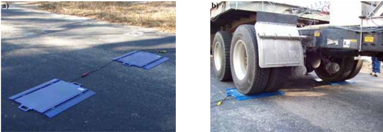
Figure 7.1. Axle load measurement: a) two portable scales, b) forward axle of the rear tandem of the truck tractor during the measurement
