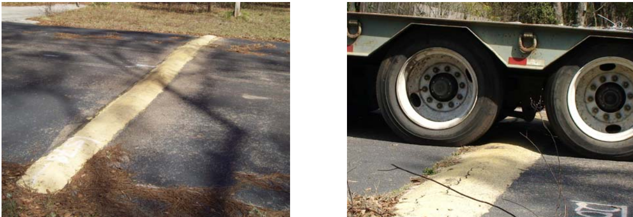
Figure 4.15. A speed bump used for the suspension tests for the tractor-trailer and the crane
