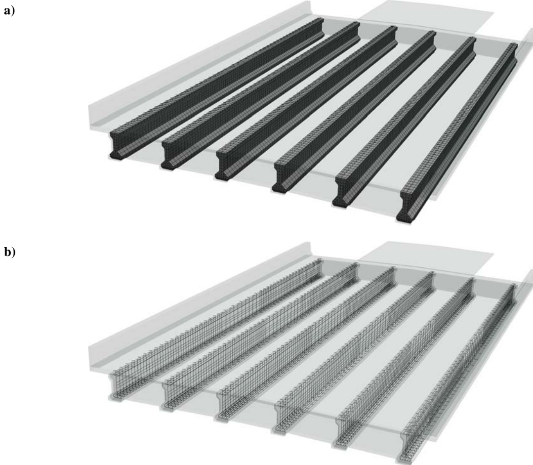
Figure 4.6. FE model of the beams: a) concrete, b) reinforcing bars and strands
