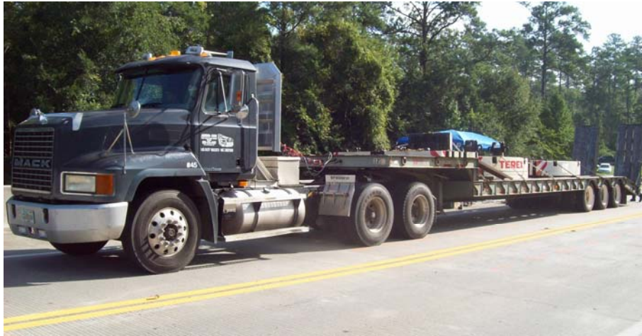
Figure 3.7. Mack CH613 truck tractor with a three axle single drop lowboy trailer used in the tests
