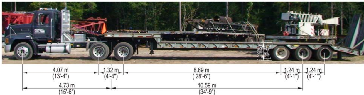
Figure 4.18. Truck tractor and lowboy trailer used in the tests
