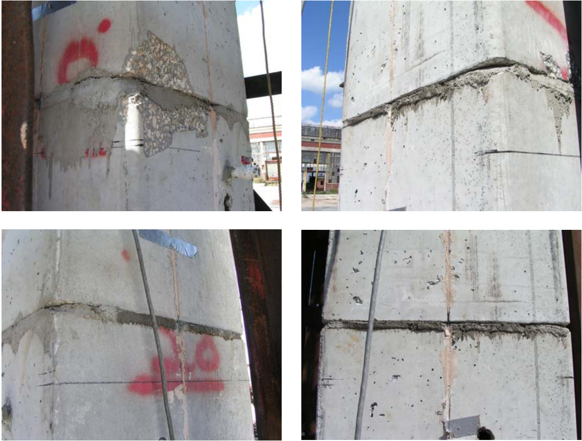
Figure 2-7 Set 45 grout used to seal mating surface after curing 45 minutes.
